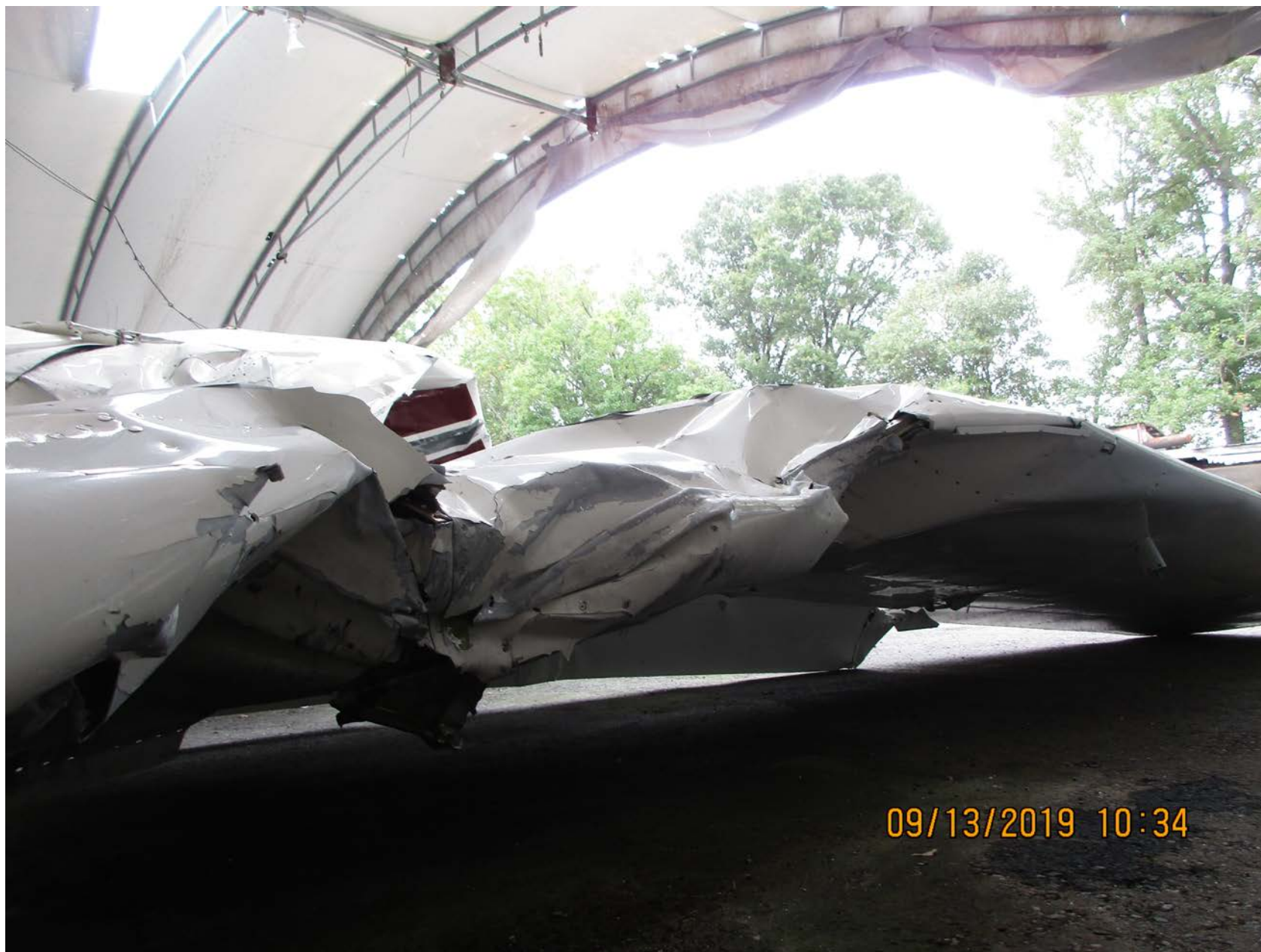
Photo 8 – Leading edge damage to left wing (Courtesy of FAA)
