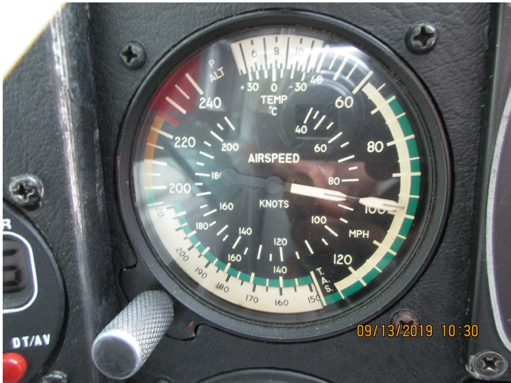
Photo 5 – View of airspeed indicator in post-accident uncalibrated test.
