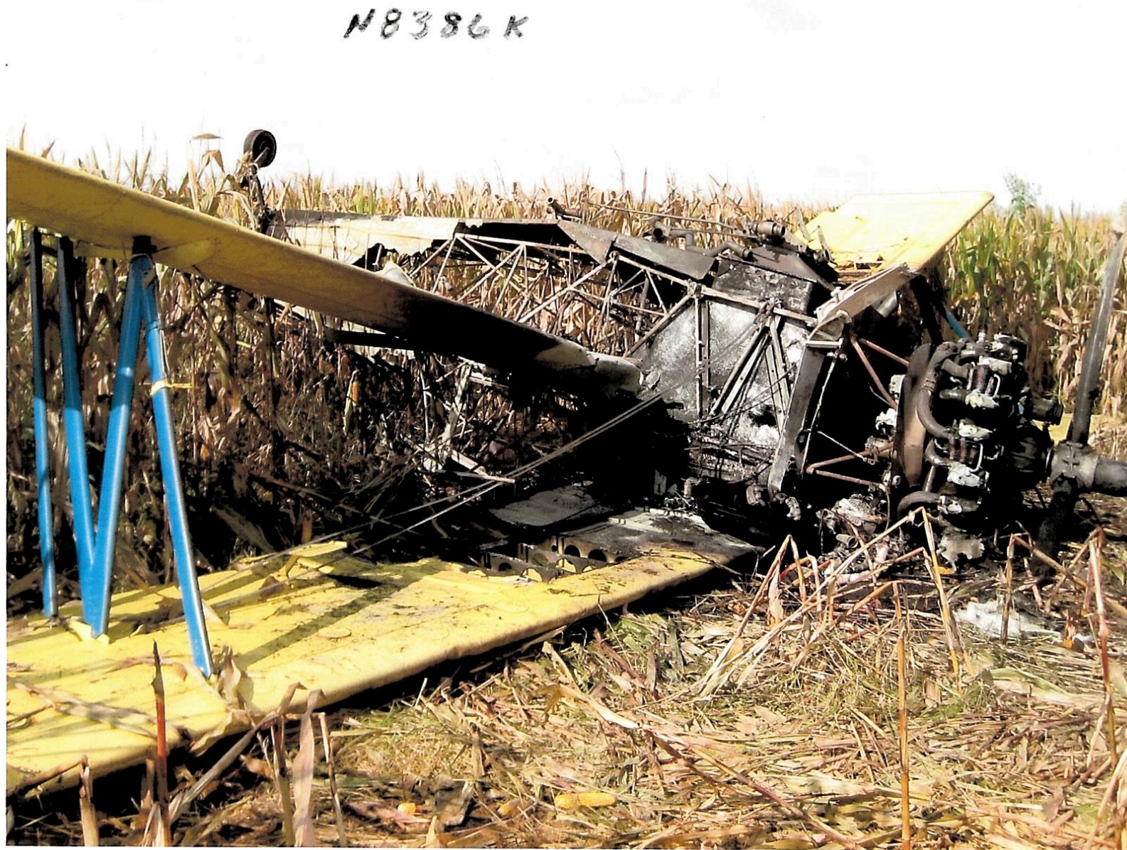
Photo 1 – View of airplane inverted and fire damaged
