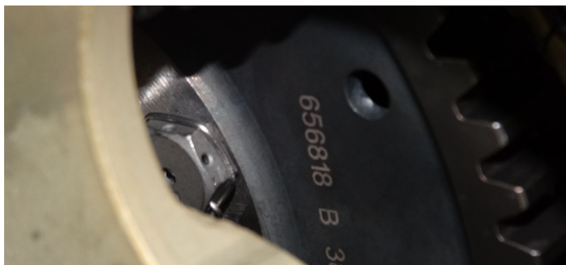
Figure 1. Camshaft Gear Part Number Location, typical (P/N is visible through the starter adapter mounting pad opening)
