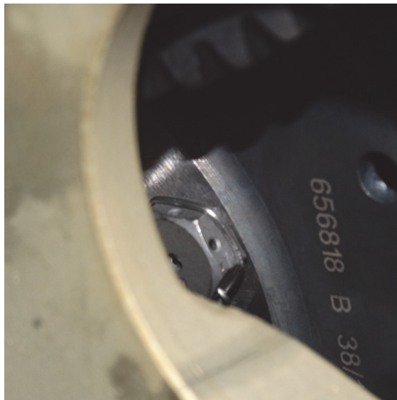
Figure 2. Camshaft Gear Part Number Location, typical (P/N is visible through the starter adapter mounting pad opening)
