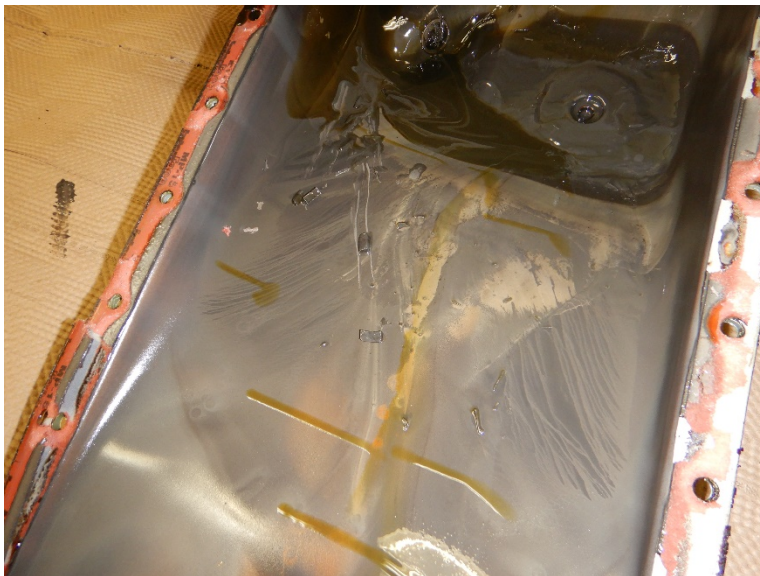
Figure 3: Sheered Teeth in Oil Pan
