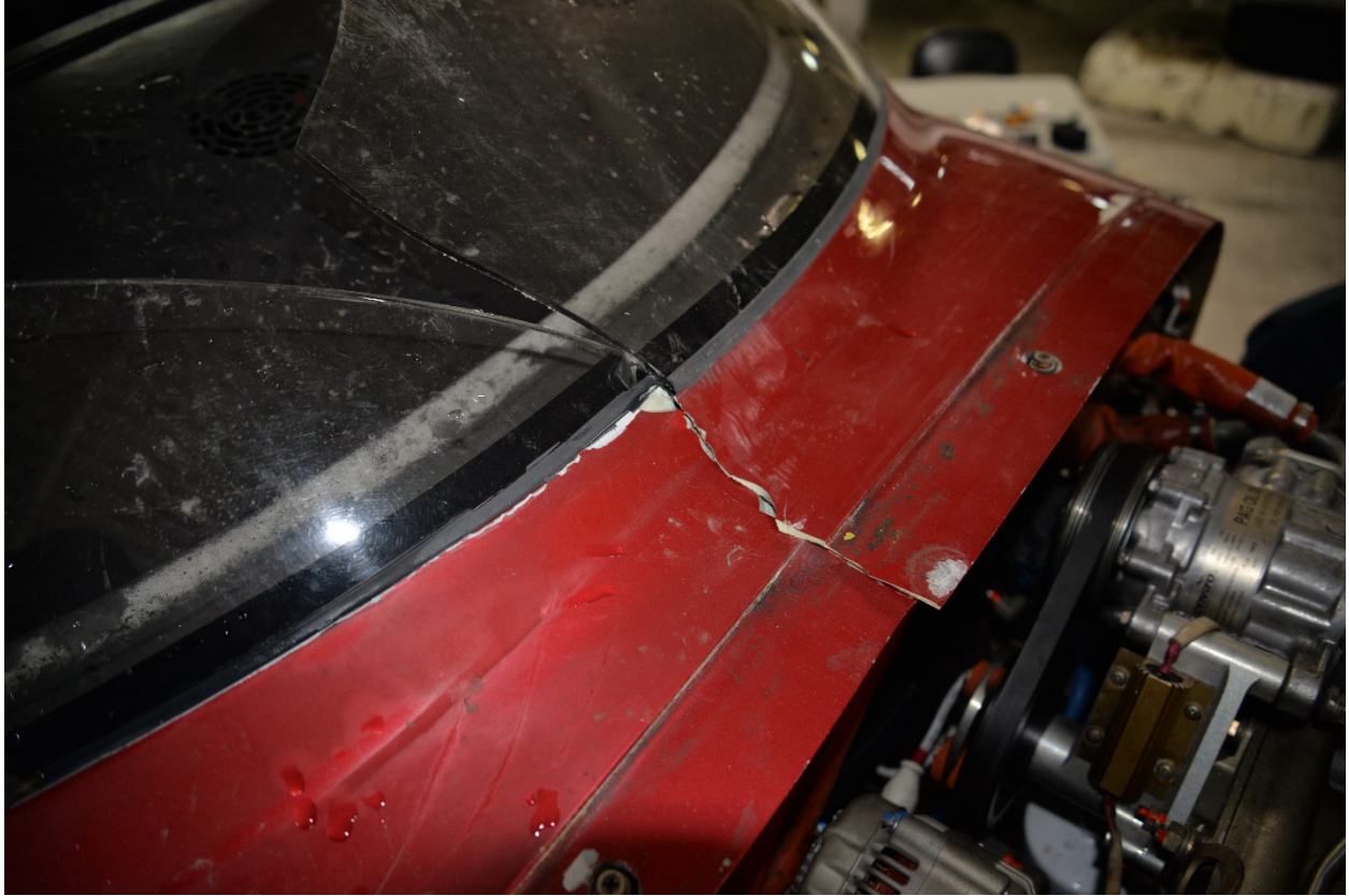
Figure 1: Fuselage fracture at center bond line (Photo Courtesy of Cirrus)
