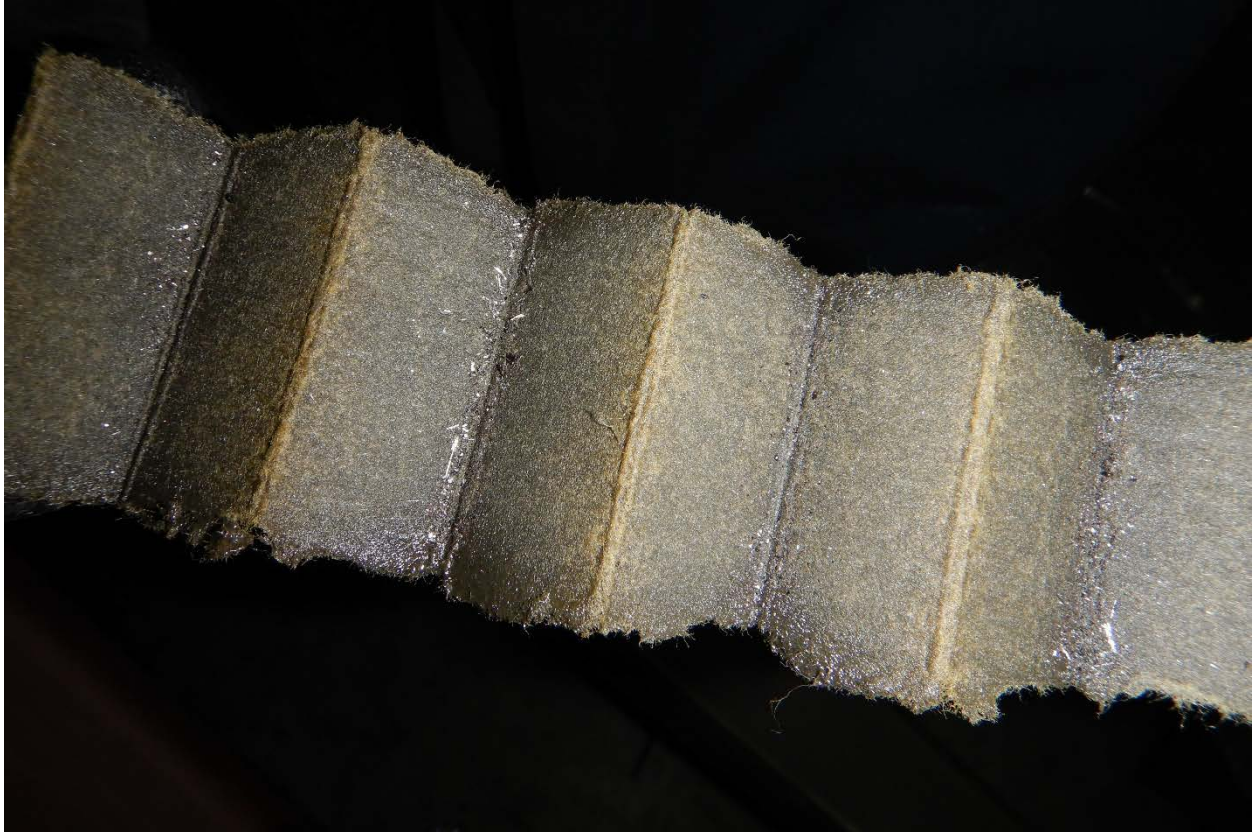
Figure 11: Metal Shavings on Oil Filter
