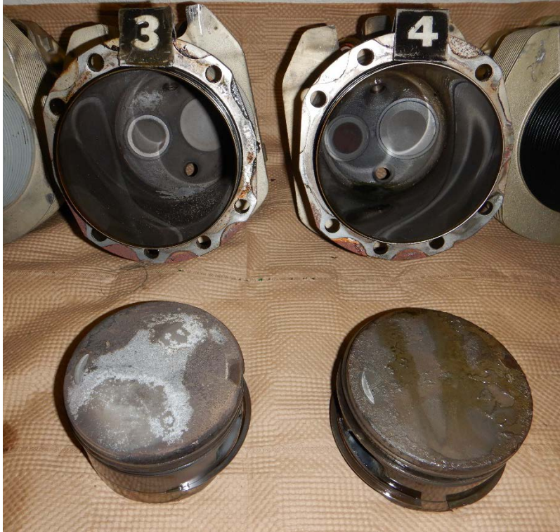
Figure 6: Valve Strikes on Pistons Nos. 3 and 4
