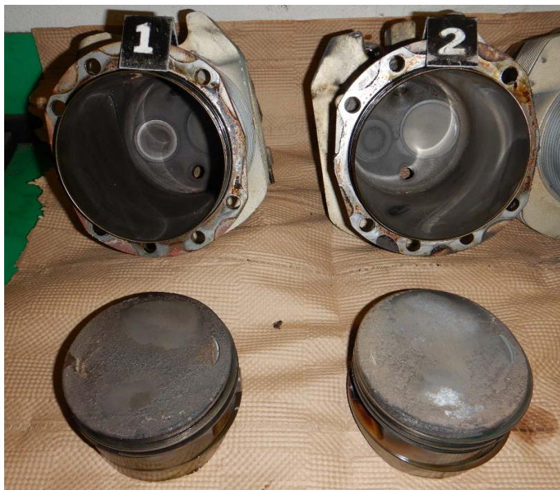
Figure 5: Valve Strikes on Pistons Nos. 1 and 2
