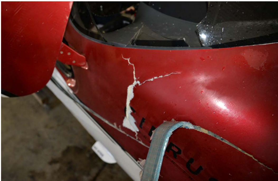
Figure 2: Fuselage crack above right CAPS harness attach fitting (Photo Courtesy of Cirrus)
