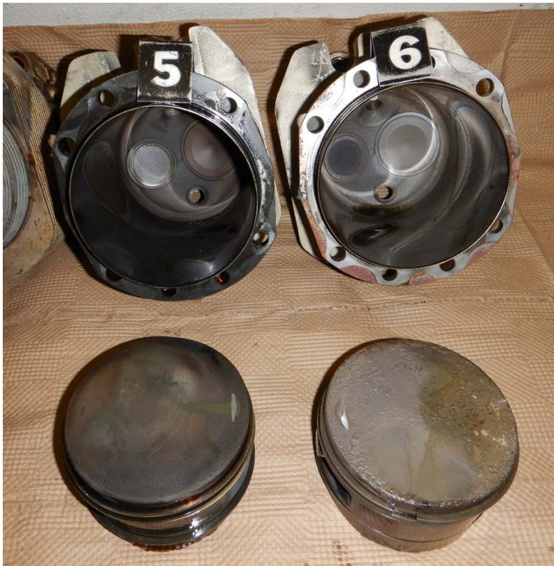
Figure 7: Valve Strikes on Pistons Nos. 5 and 6
