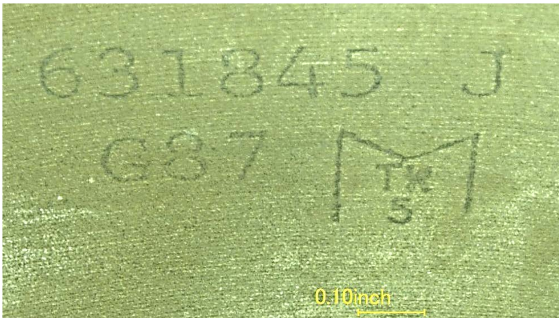
Figure 2. Photograph of the part number "631845" found on the forward face of the camshaft gear.
