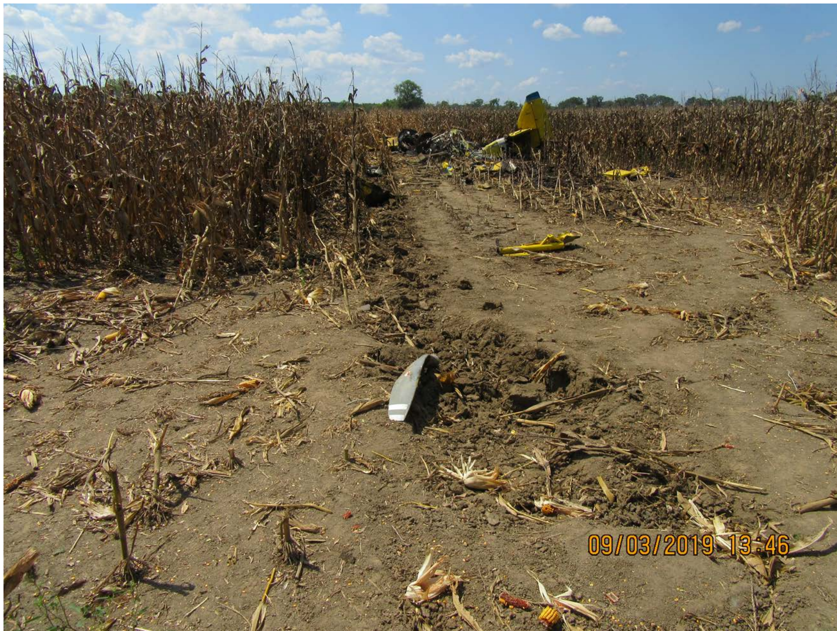
Photo 4 – Separated Propeller Blade (FAA Photo)
