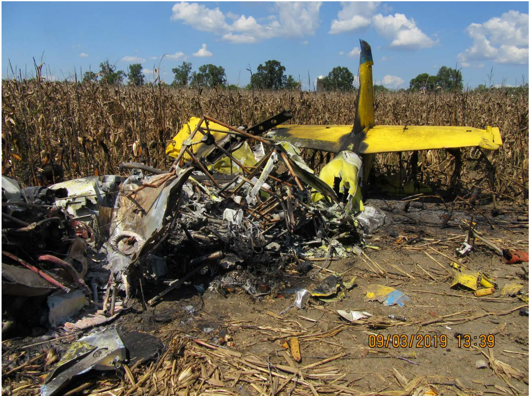
Photo 1 – Aft Fuselage and Empennage (FAA Photo)
