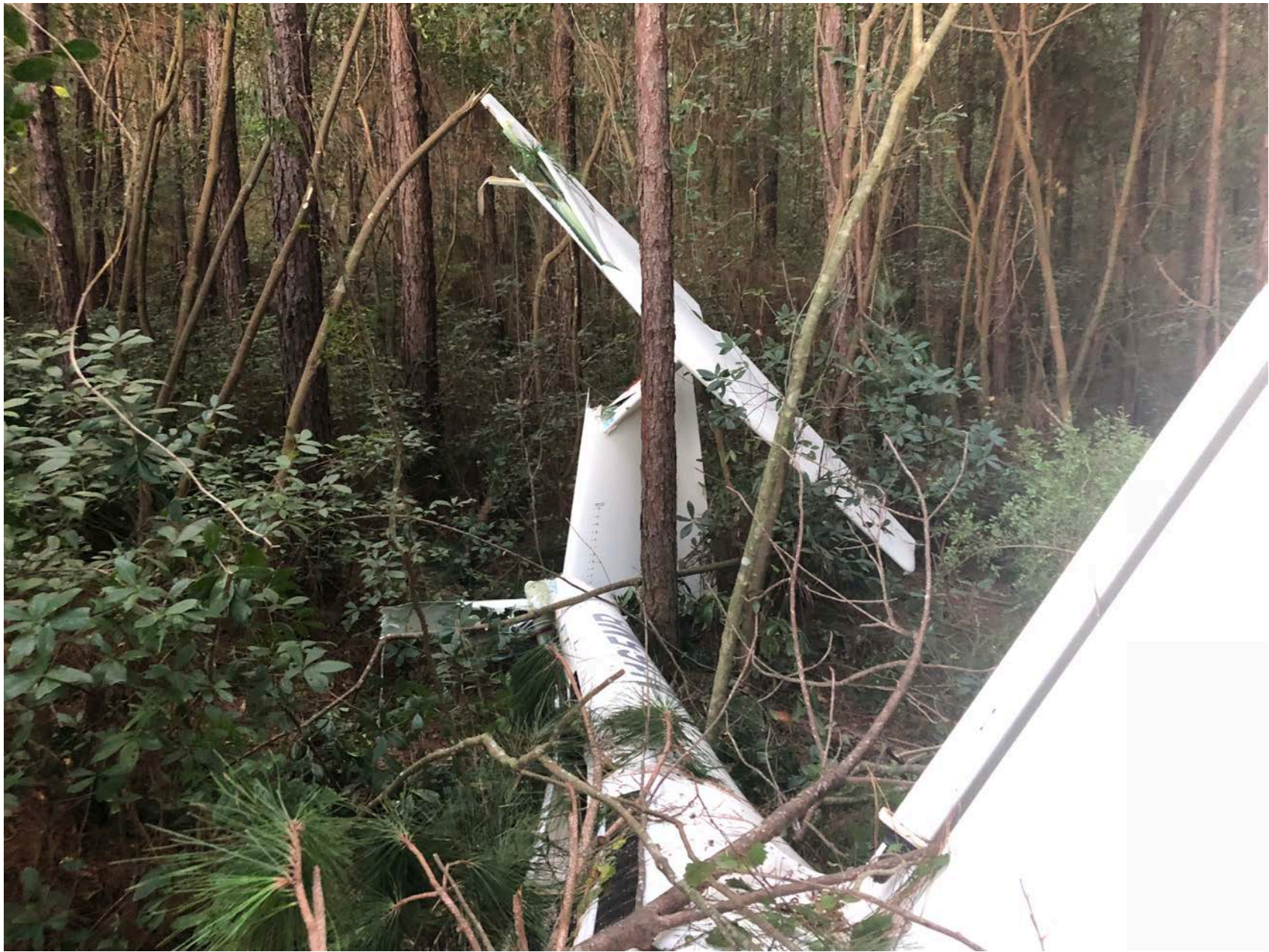
Photo 4 - Empennage (FAA Photo)
