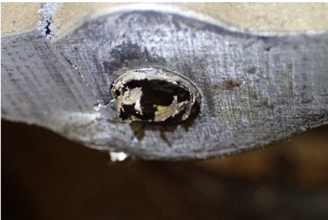
Sealant found on crankcase mating surfaces
