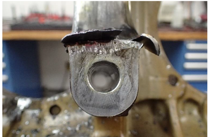
Left Side #2 Bearing Support Mating Surfaces
