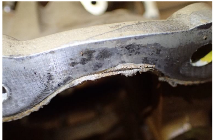
Sealant found on crankcase mating surfaces
