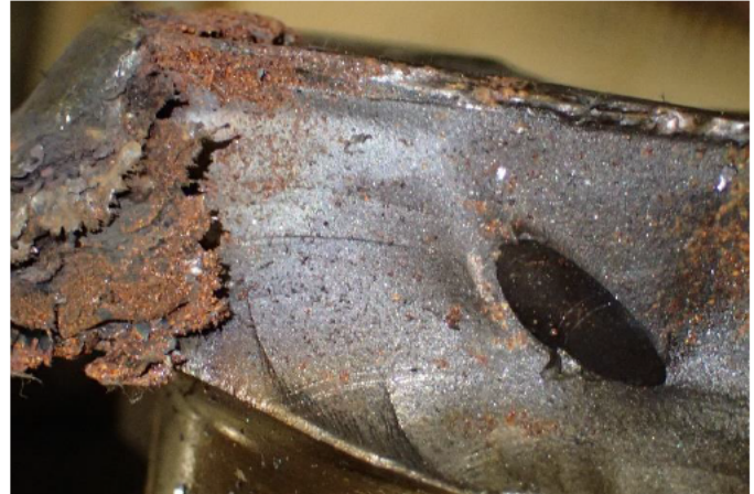
Fracture Surface on Aft Portion of the Crankshaft
