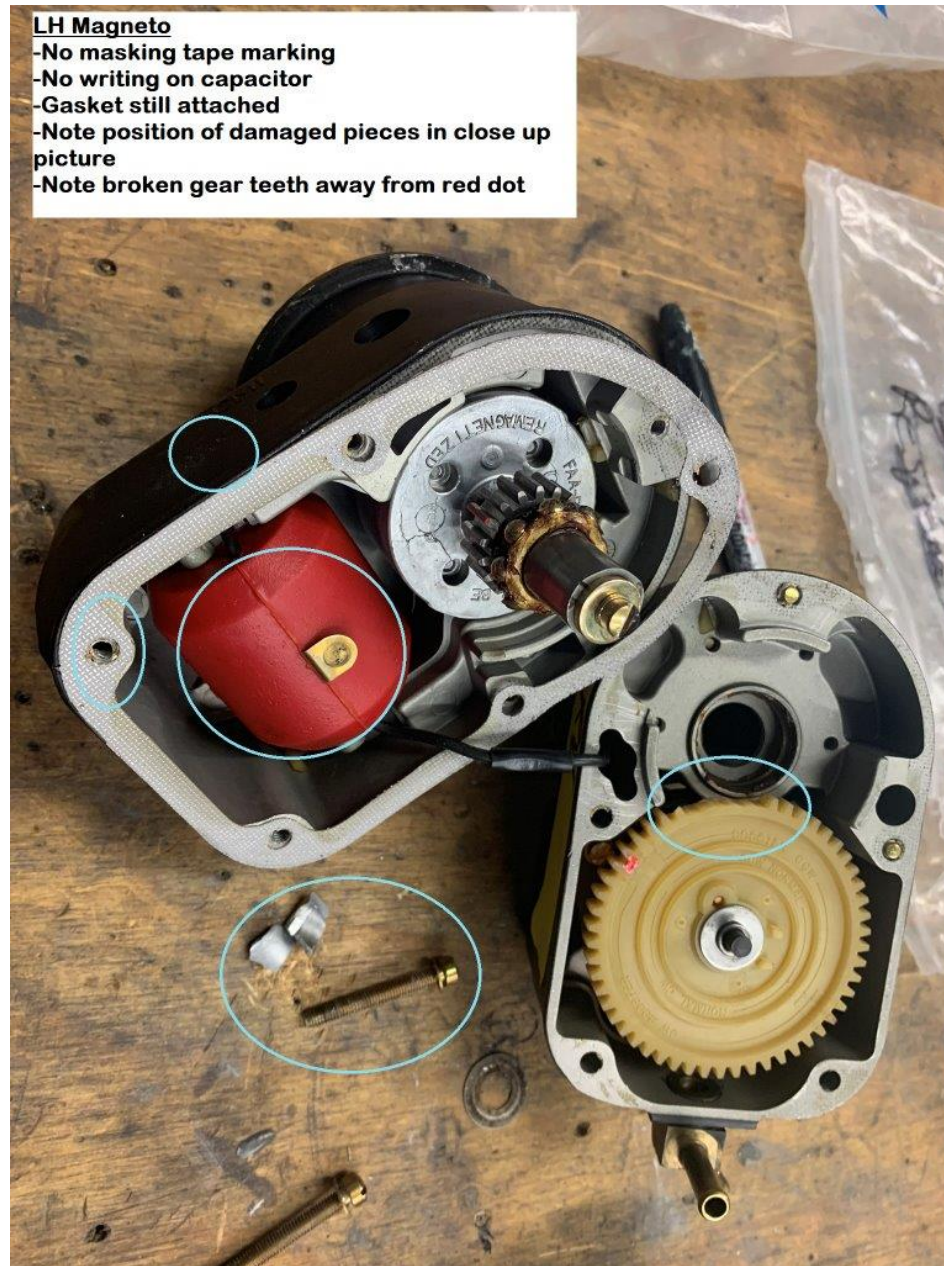
Photo 3 – View of Left Magneto During Disassembly (Myers Aviation)
