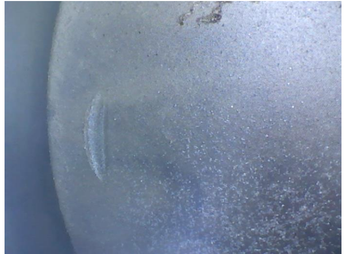
#3 Piston (with indentation consistent with a valve strike)
