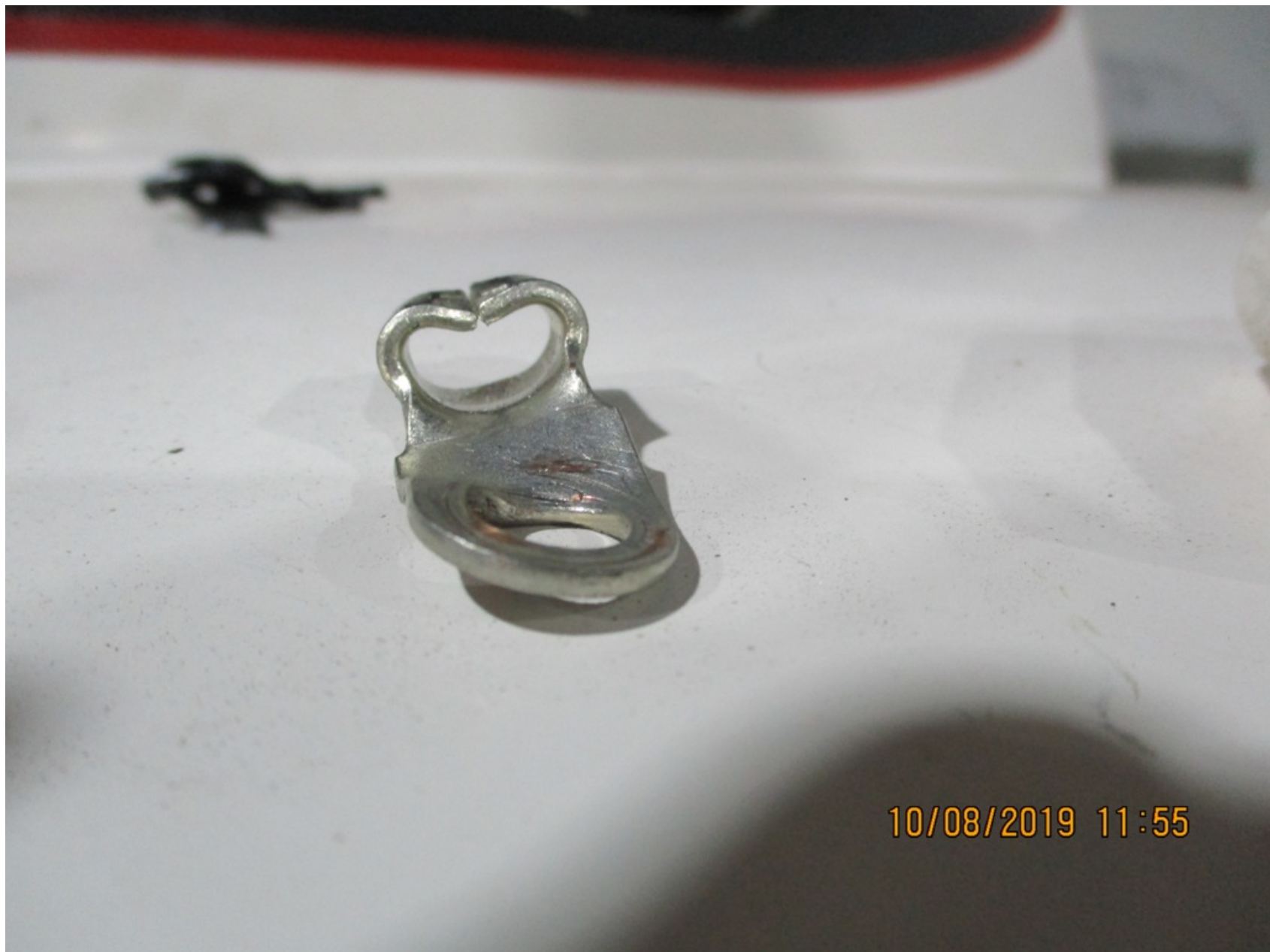
Photo 6 - Negative Battery Lead Connector (Photo NTSB)
