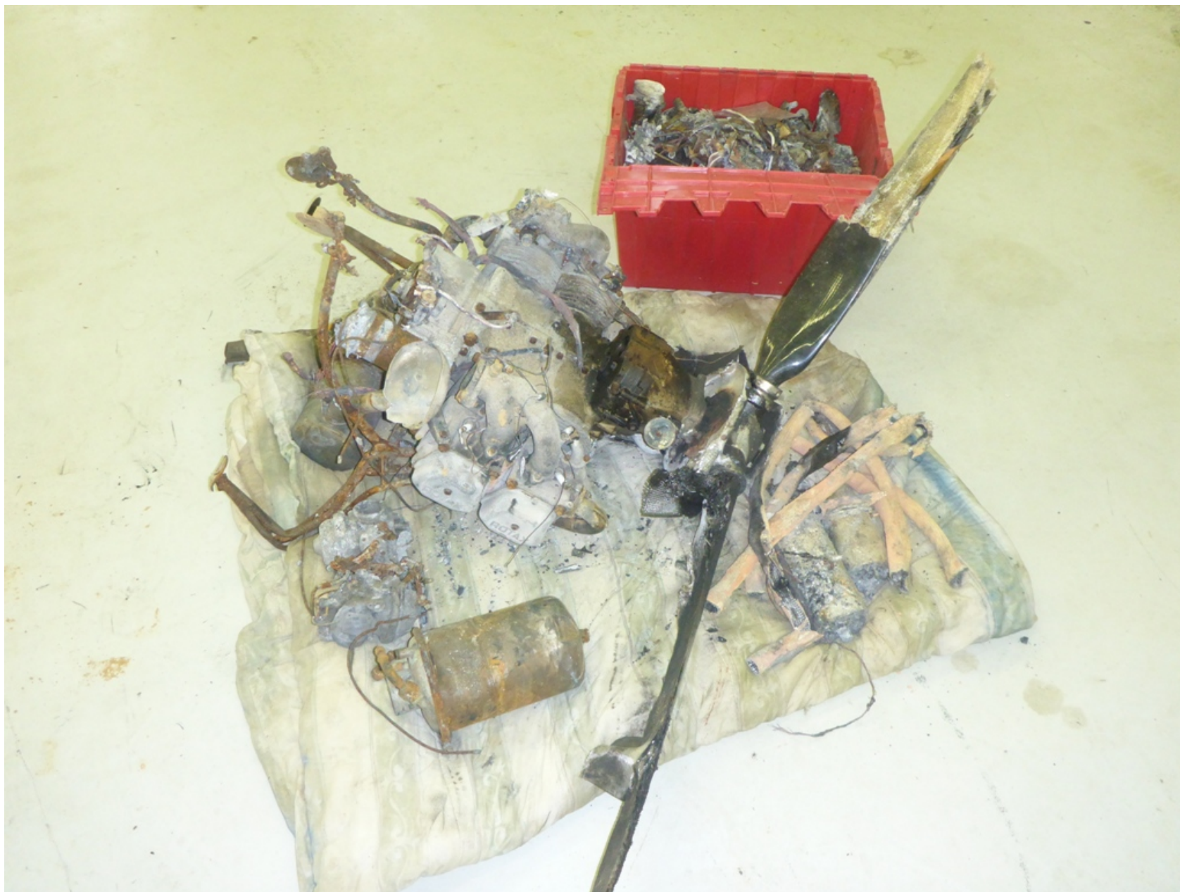
Photo 6 – Rotax Digital Photograph. Right Side View of the Engine and Propeller Assembly Following Recovery. Note the Extensive Fire Damage.
