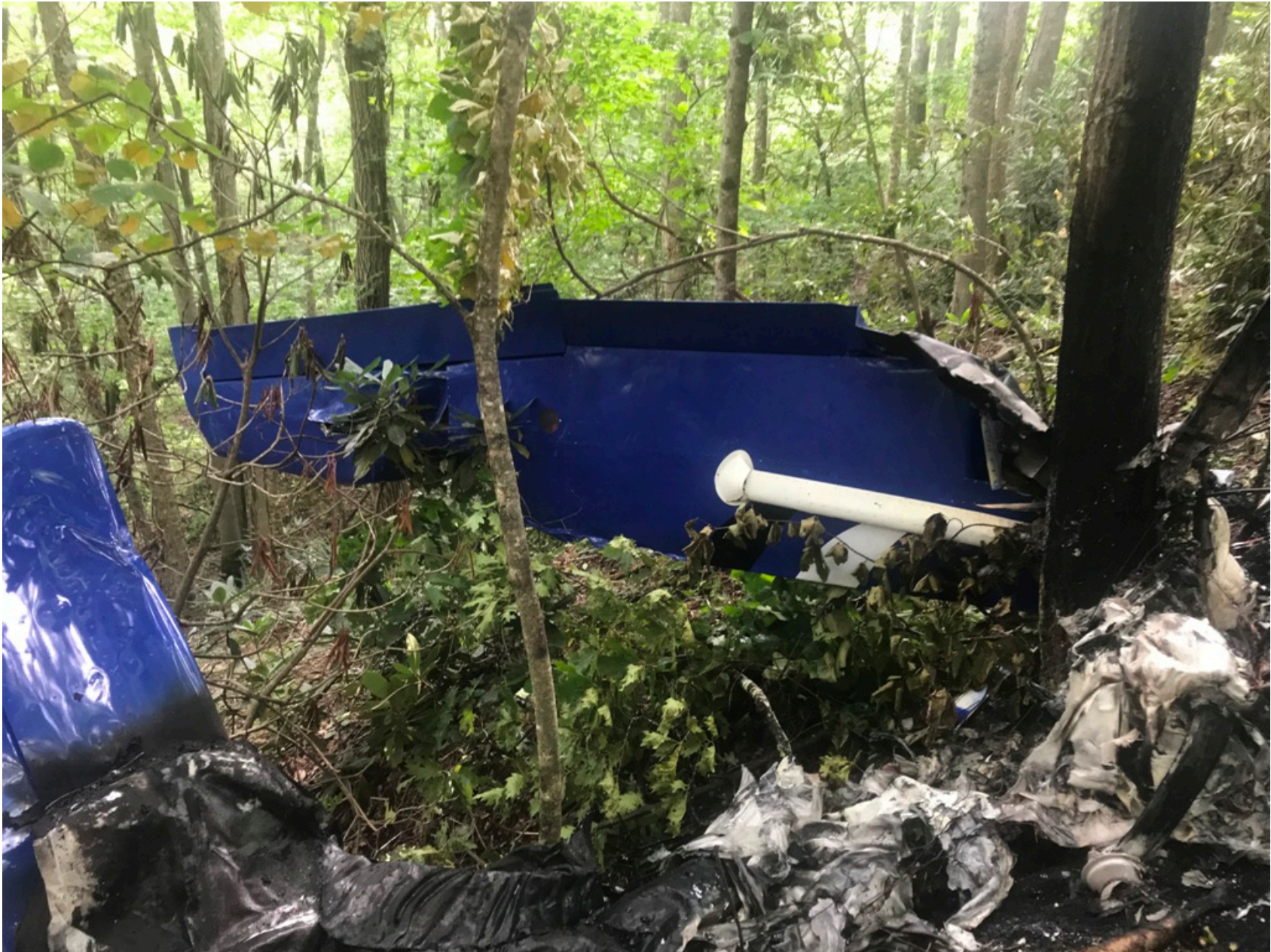
Photo 2 – NC State Highway Patrol Photograph. Aft Side View of the Left Wing. Note the Impact Damage to the Leading Edge.
