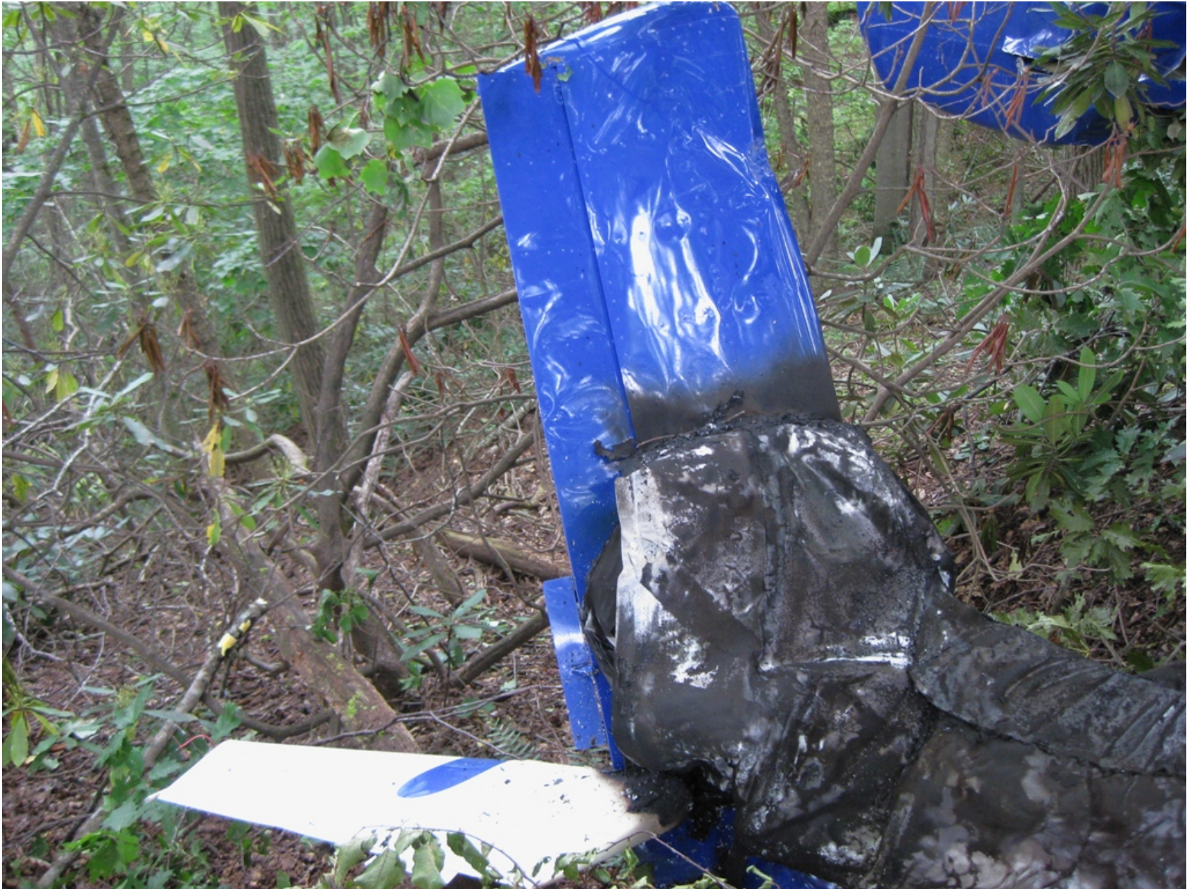
Photo 4 - FAA Digital Photograph. Right Side View of the Upper Portion of The Vertical Stabilizer, Right Stabilizer and Elevator, and Partially Attached Rudder.
