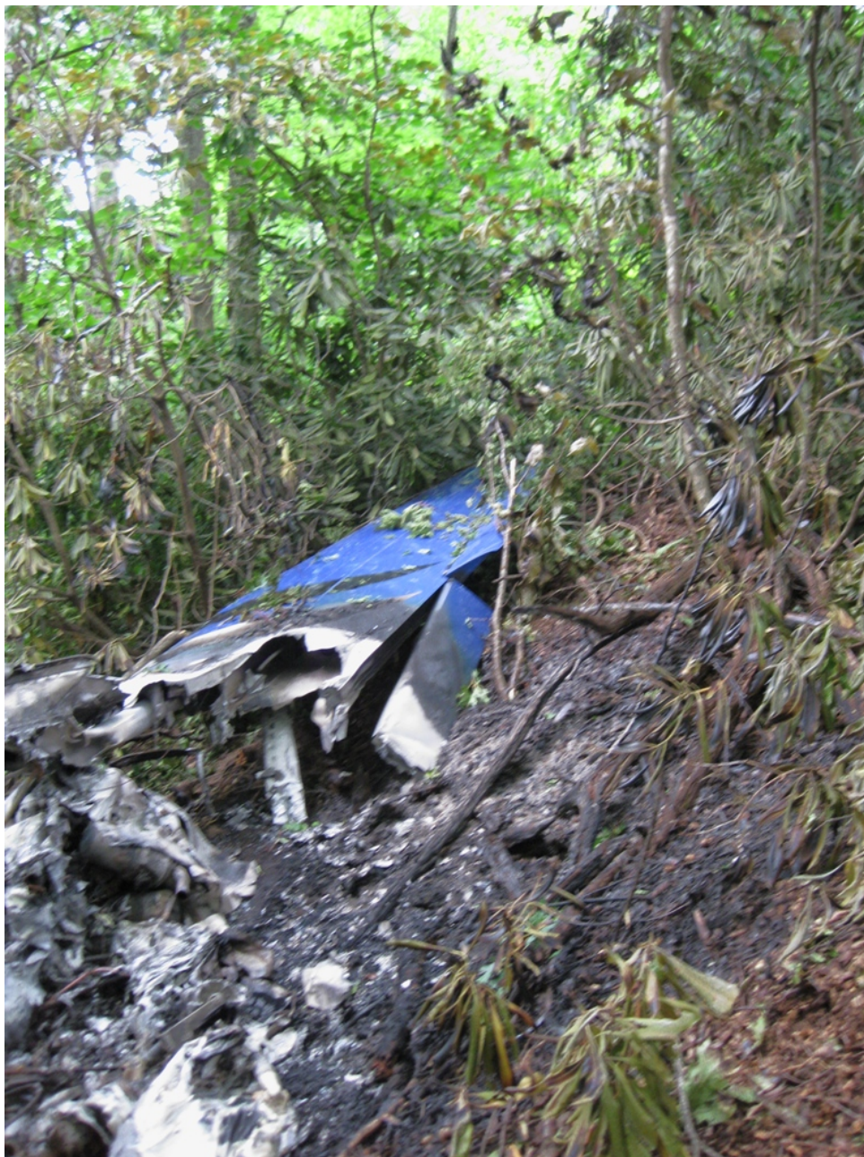
Photo 3 - FAA Digital Photograph. Aft Side View of the Right Wing. Note the Fire Damage to the Inboard section of the Wing.
