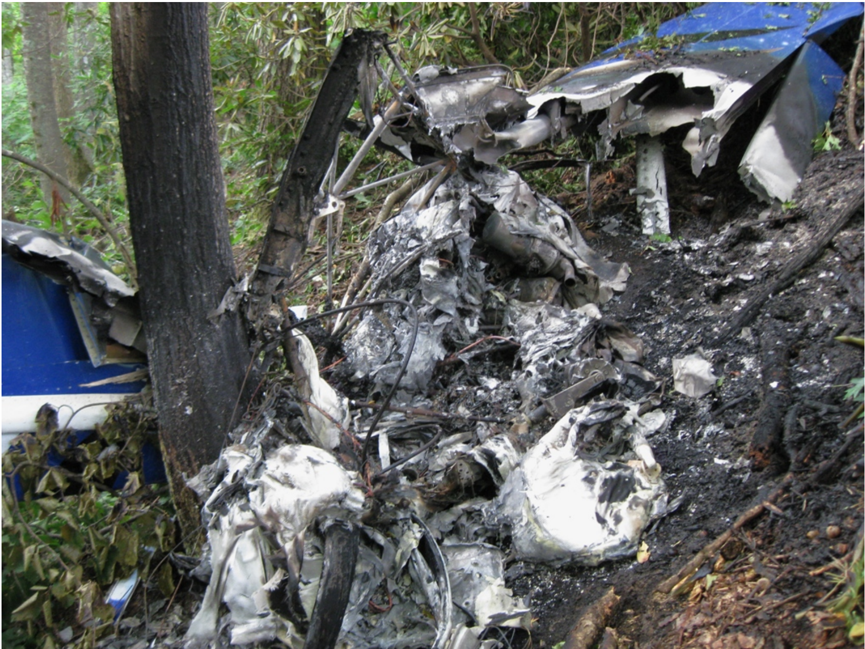
Photo 5 - FAA Digital Photograph. View of the Cockpit. Note the Extensive Fire Damage.
