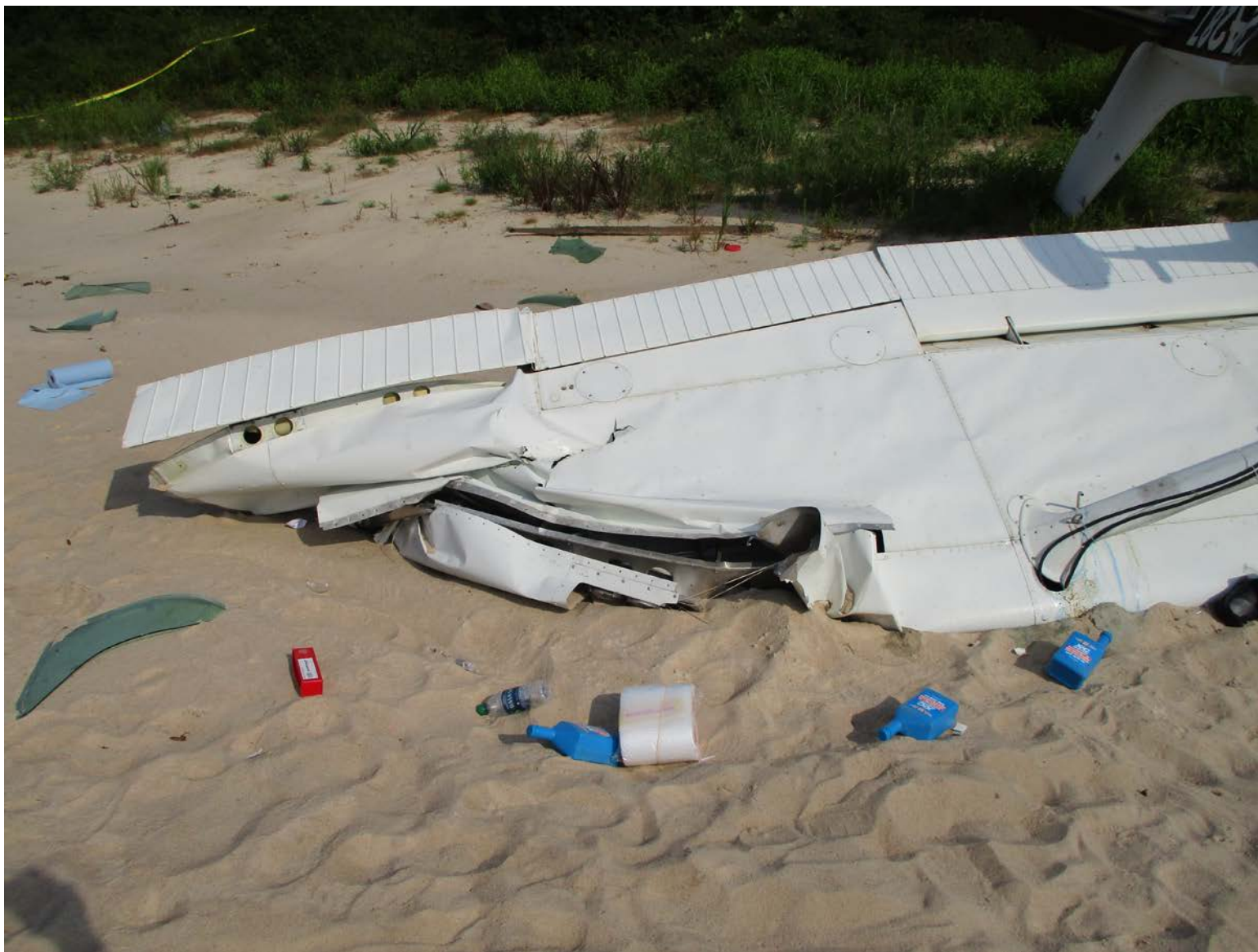
Photo 2 – Close up view of left wing damage. (Courtesy of FAA)
