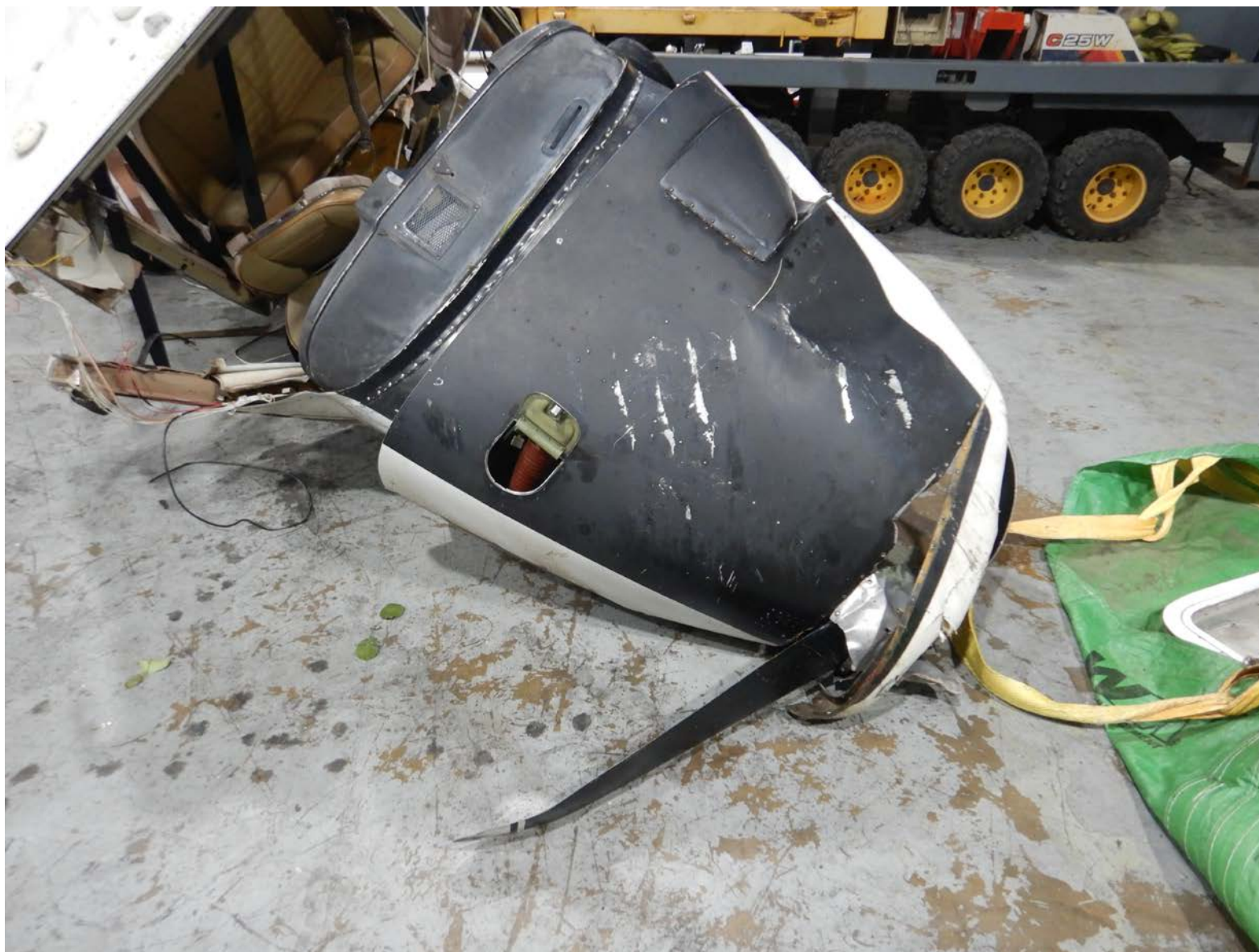
Photo 5 – Top of engine cowl and propeller damage. Note the six polished scrapes in the paint. (Courtesy of Lycoming)
