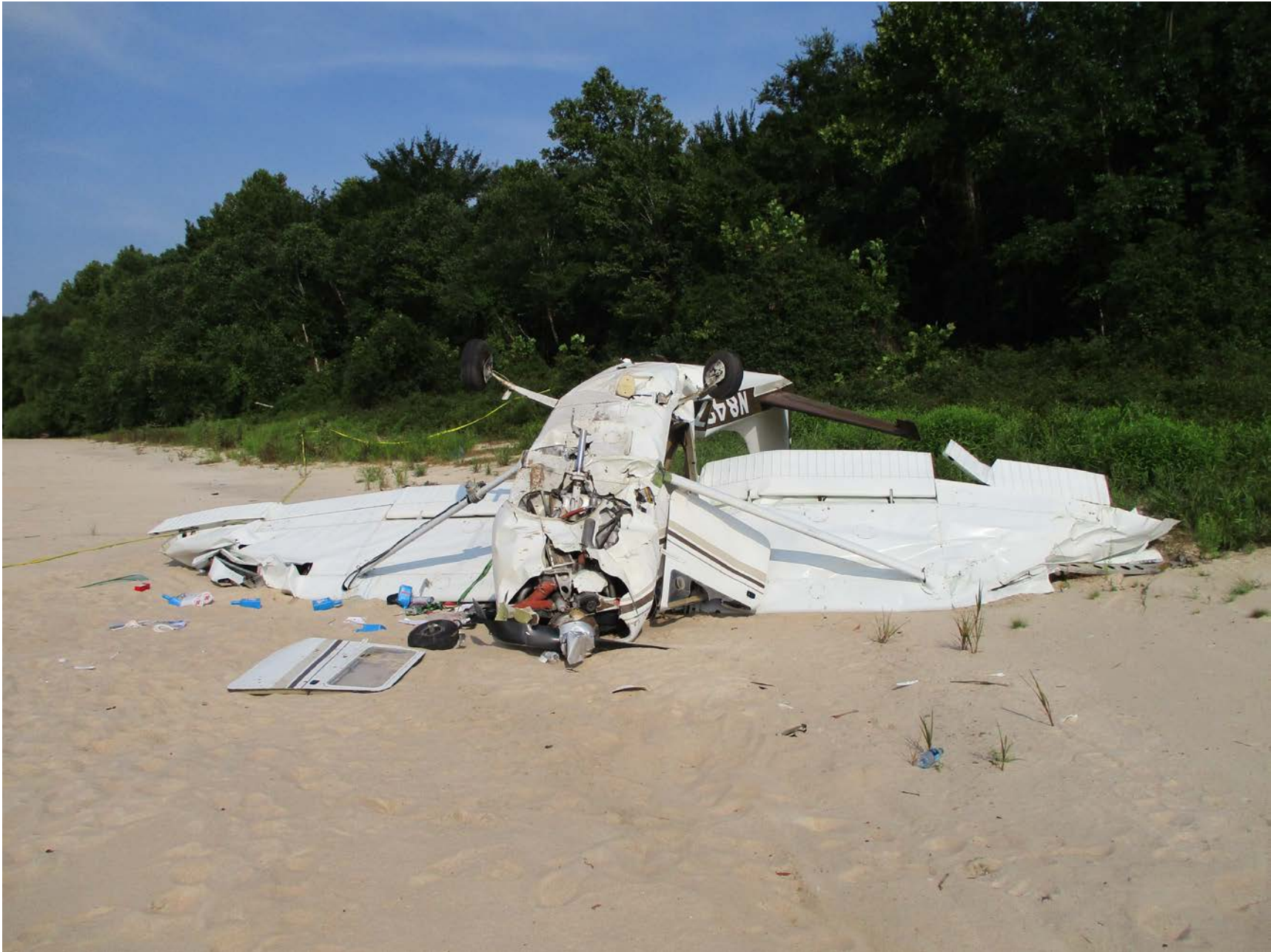
Photo 3 – Airplane inverted on the sandbar showing damage to both wings and fuselage. (Courtesy of FAA)
