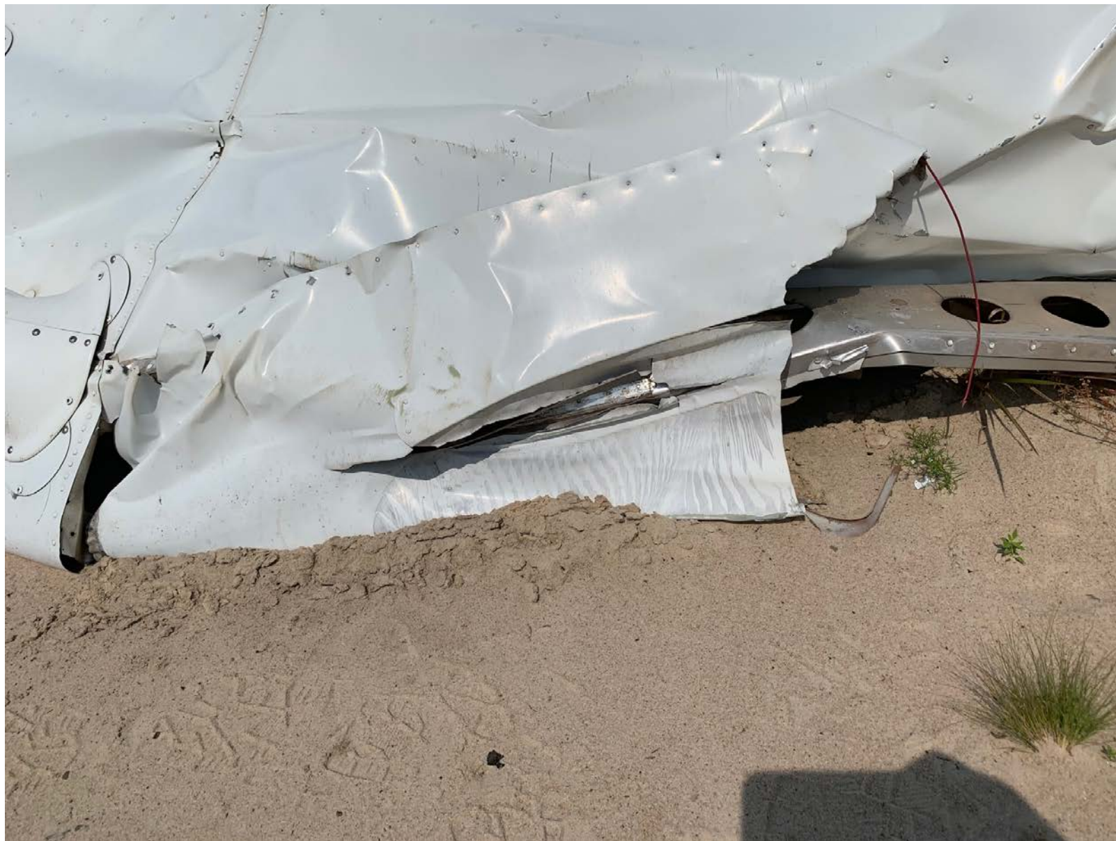
Photo 4 – Close up view of right wing leading edge damage. Note powerline polishing & scrape marks. (Courtesy of FAA)
