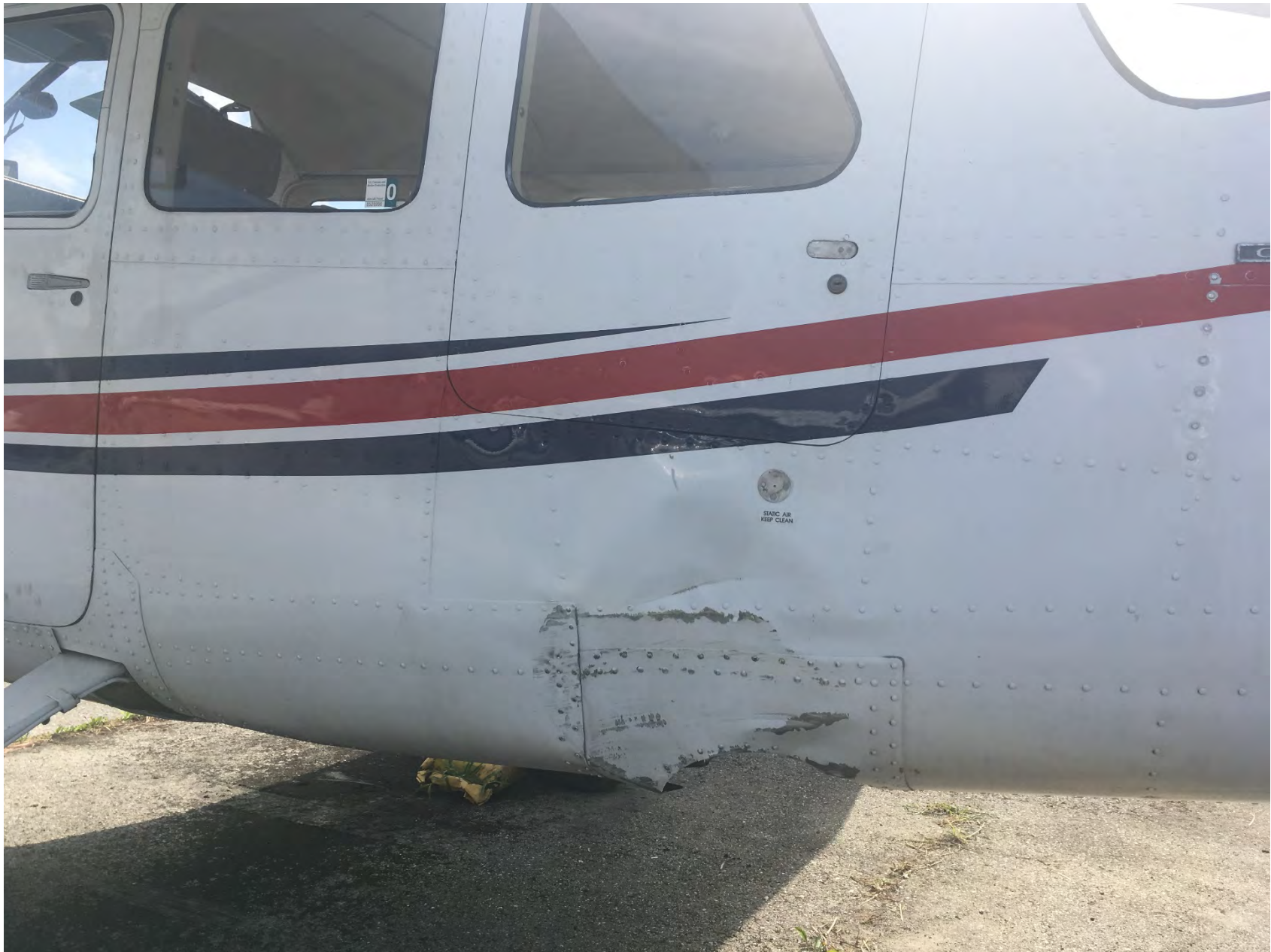
Photo 7 – Close-up View of Fuselage Damage (Photo Courtesy of FAA)
