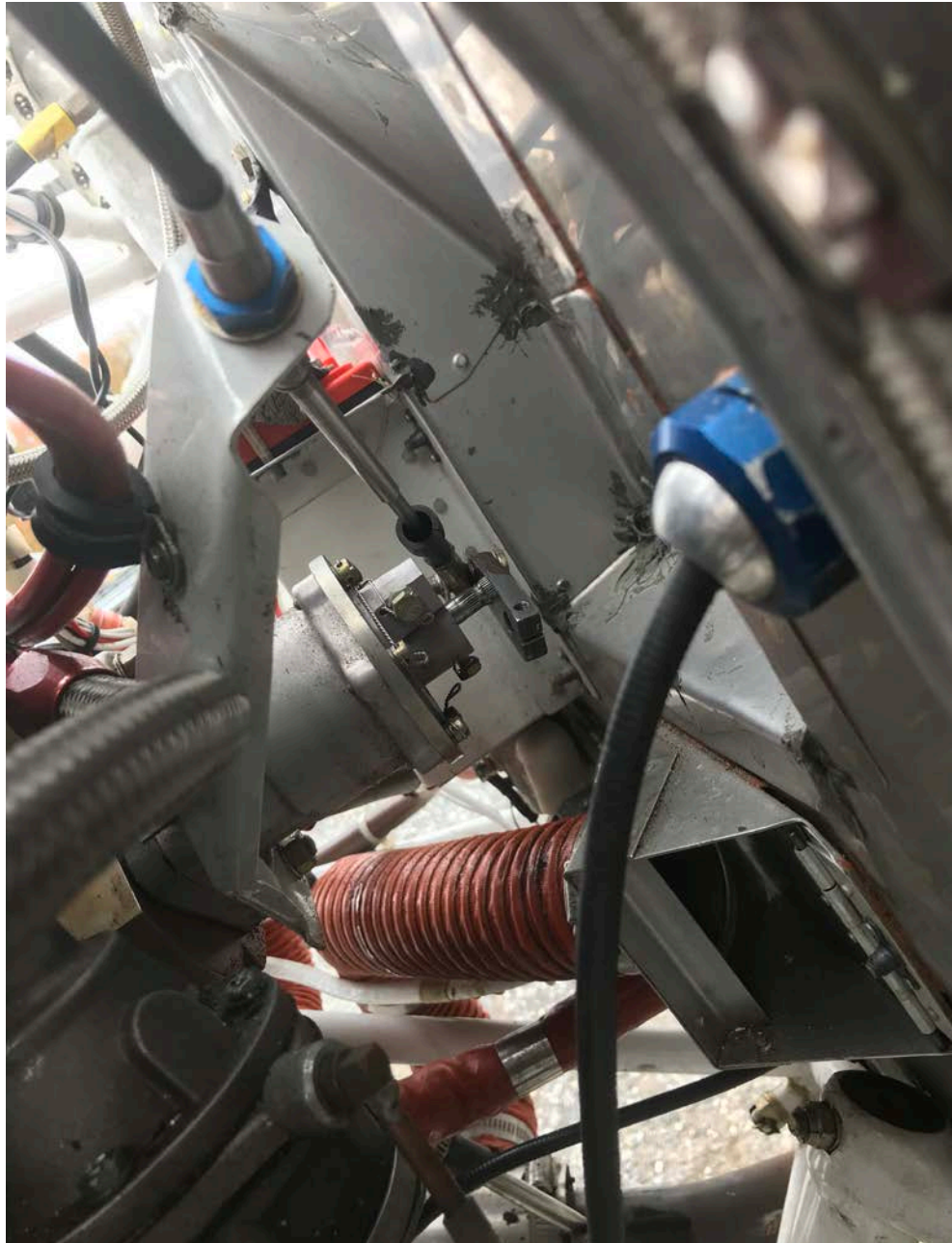
Photo 3 – View of control arm separated from propeller governor.
