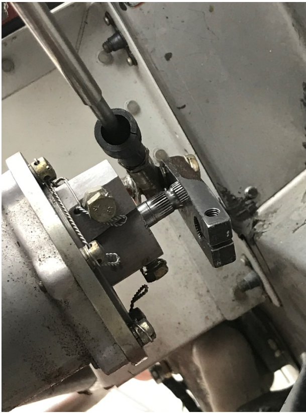
Figure 3. View of control arm not attached to propeller governor.
