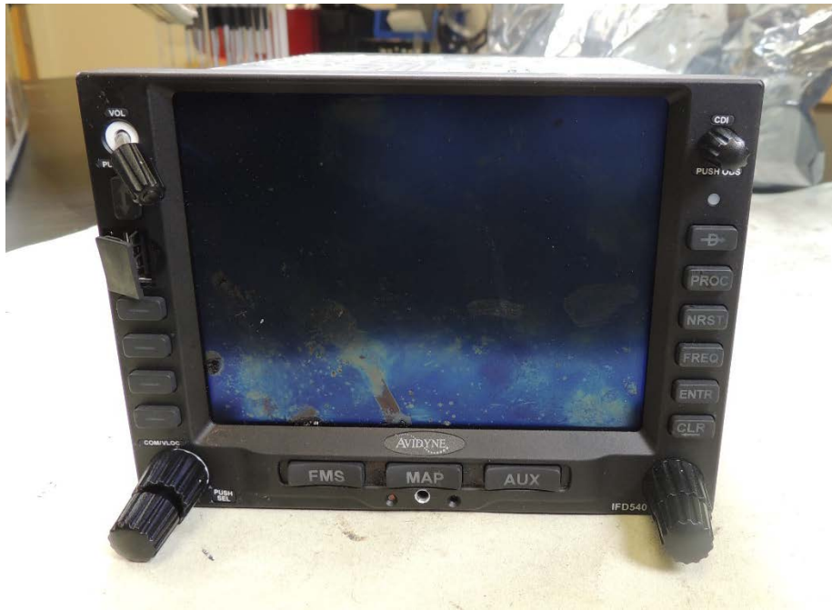
Figure 1. Exterior damage to IFD 540 (device 1)
