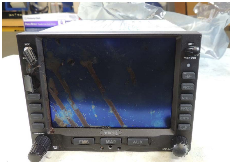
Figure 2. Exterior damage to IFD 540 (device 2)
