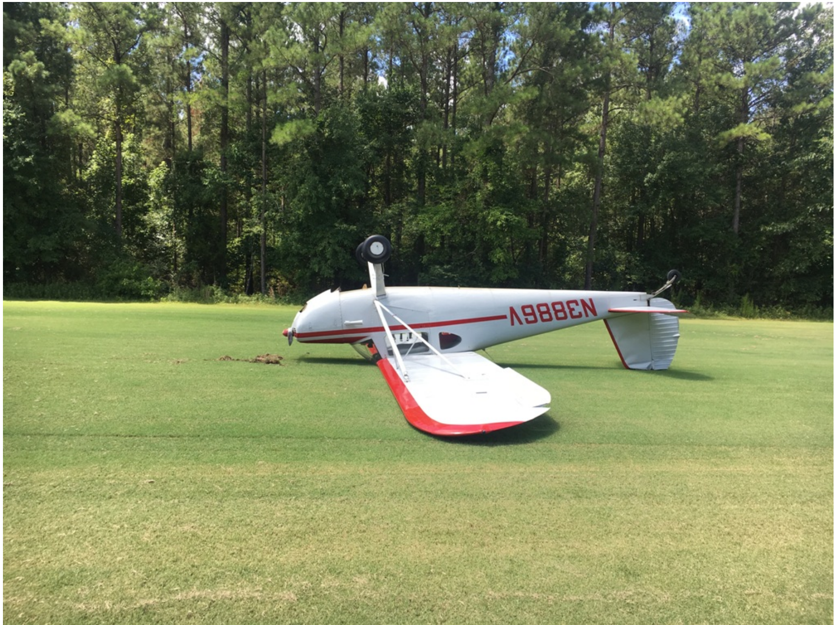
Photo 1 – Digital Photograph From Pilot. Right Side View of the Airplane At the Accident Site. Note the damage to the Vertical Stabilizer and Rudder.
