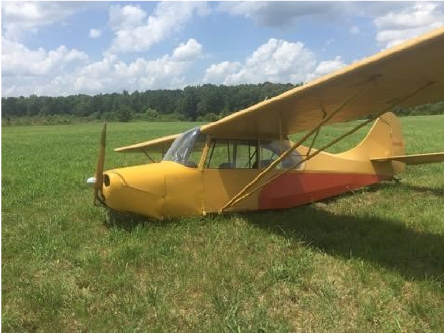
Photo 1 – View of left side of airplane showing collapsed gear and fuselage damage. (Courtesy of FAA)
