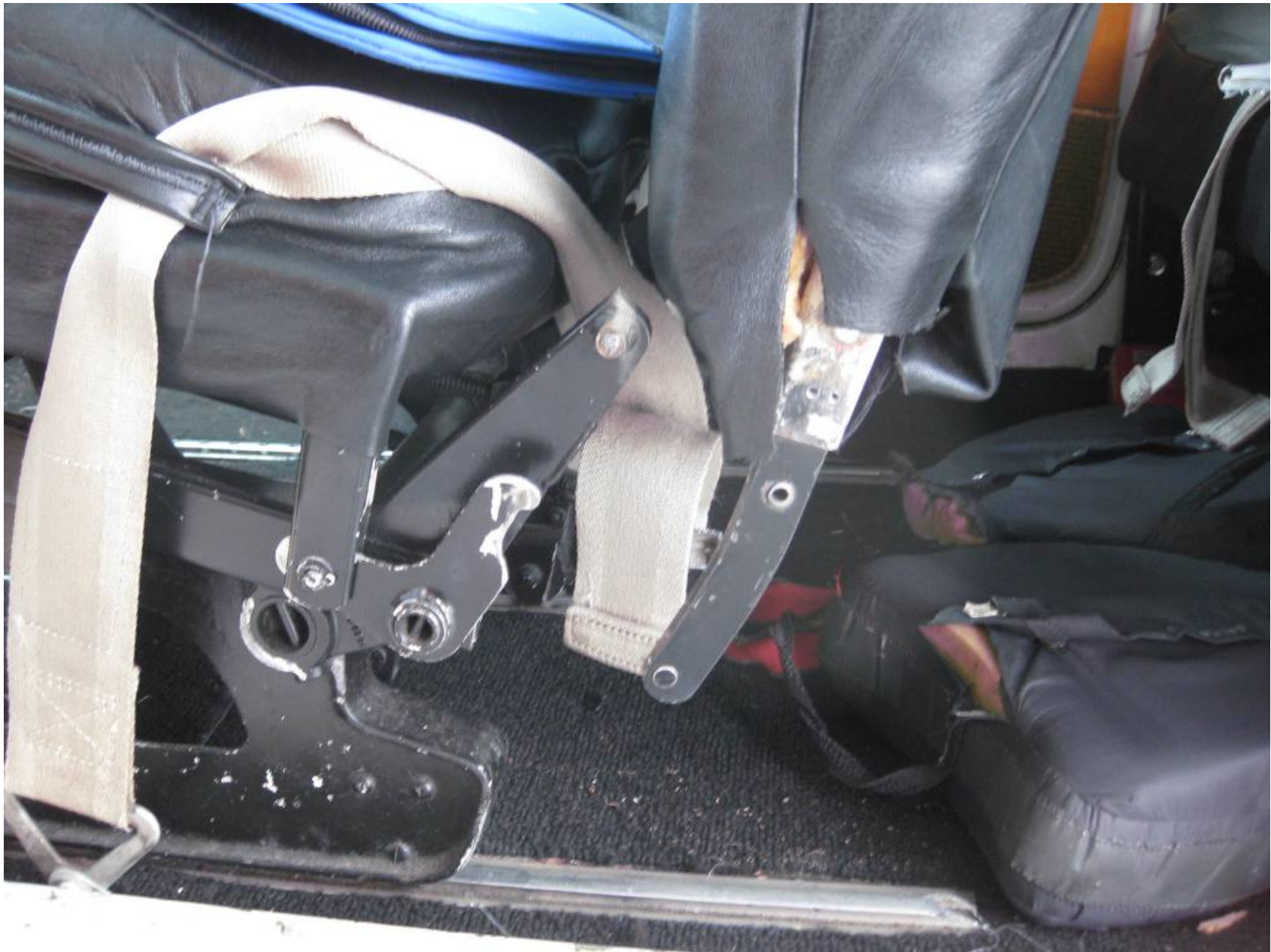
Photo 4 – Pilot's Broken Seatback courtesy of the FAA
