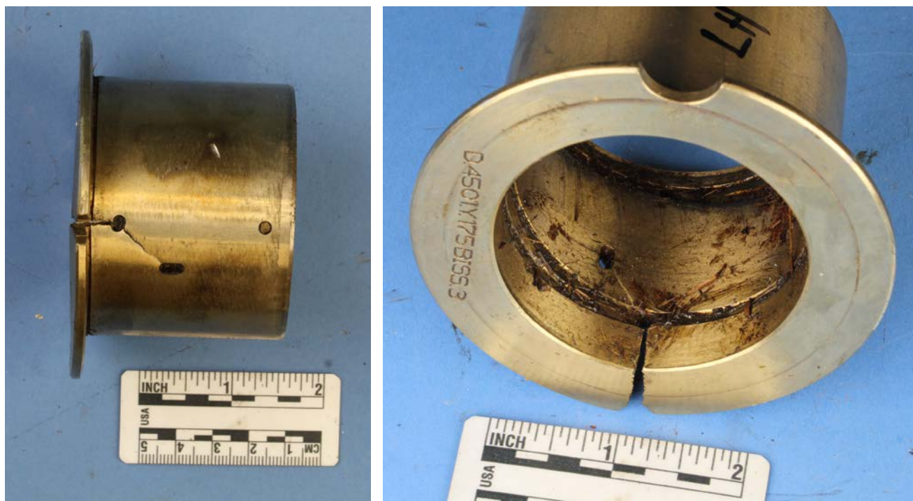
Figure 2c: Photograph of a fractured bronze bushing received with the left main landing gear. The bushing was separate from the landing gear component as-received. The crack began at a notch feature in the flange of the bushing and arrested at an elongated hole feature in the sleeve of the bushing. Plastic deformation of the flange and sleeve is apparent.
