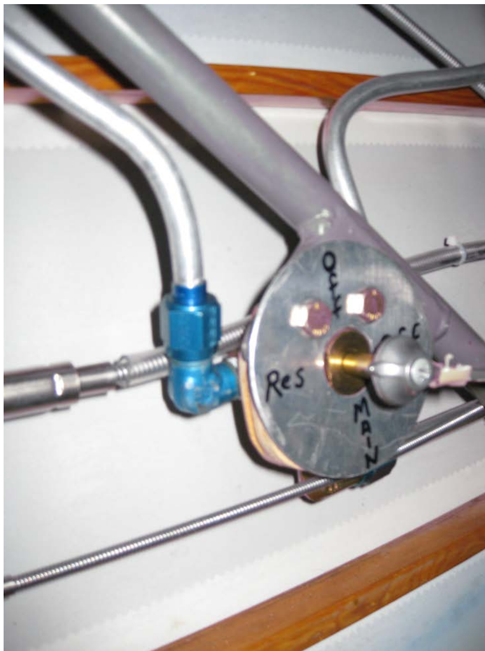
Photo 4 – View of Fuel Selector as Found (FAA)
