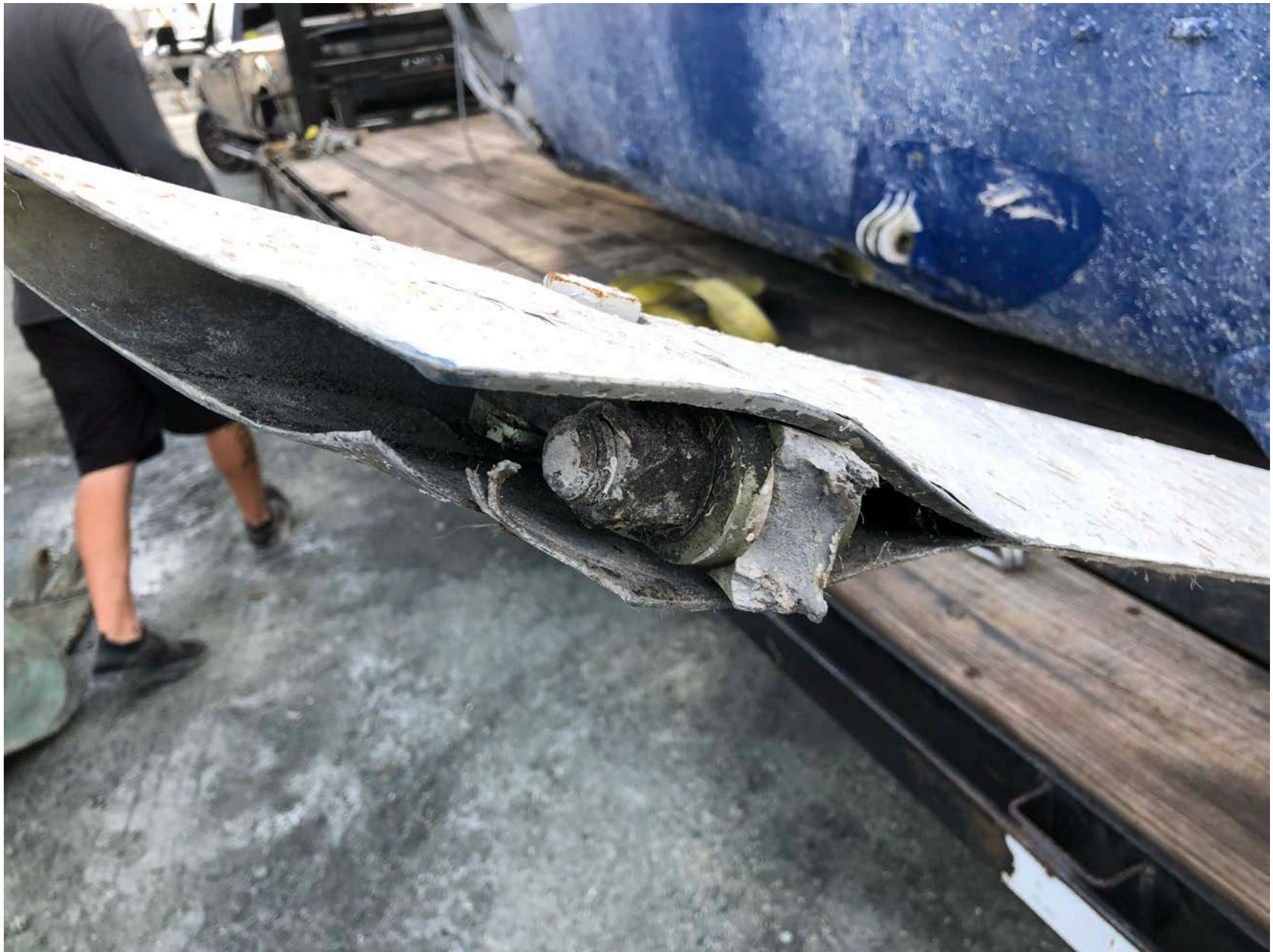
Photo 11 – Exemplar Landing Gear Attachment Hardware (Salvage Company Photo)
