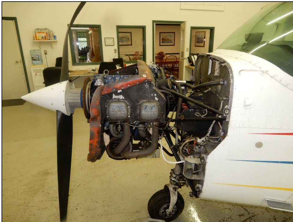
Figure 1: Overview of Engine Attached to the Firewall
