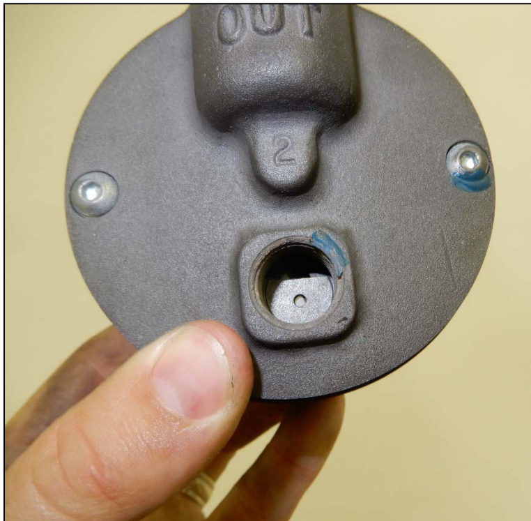
Figure 3: View of the Vacuum Pump and its Wear Indicator
