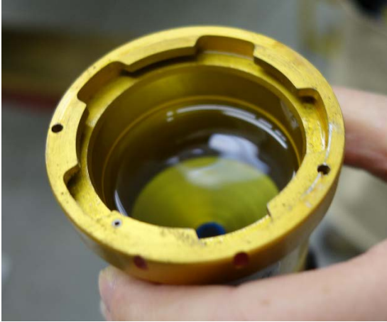
Figure 7: Fuel Strainer (Photo Courtesy of Piper Aircraft)
