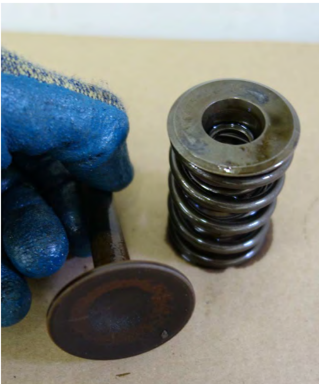
Figure 13: No. 3 Exhaust Valve and Spring (Photo Courtesy of Piper Aircraft)
