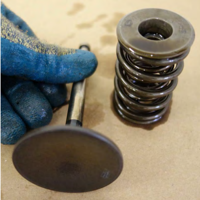
Figure 12: No. 3 Intake Valve and Spring (Photo Courtesy of Piper Aircraft)
