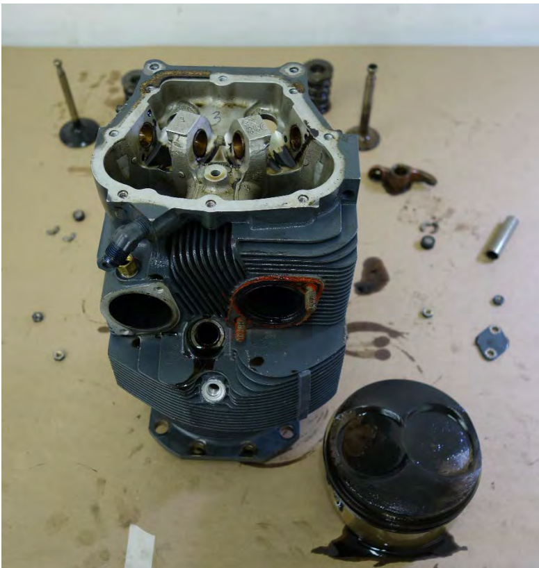
Figure 11: No. 3 Cylinder Head and Piston (Photo Courtesy of Piper Aircraft)
