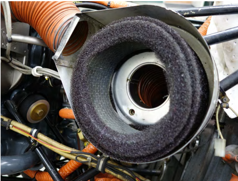
Figure 6: Air Intake and Filter Free from Obstruction (Photo Courtesy of Piper Aircraft)
