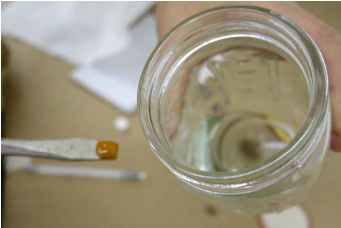
Figure 8: Fuel in Strainer Tested Free from Water (Photo Courtesy of Piper Aircraft)
