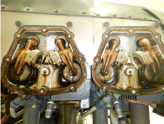
Figure 10: Rocker Covers Removed from Cylinders Nos 3 and 1
