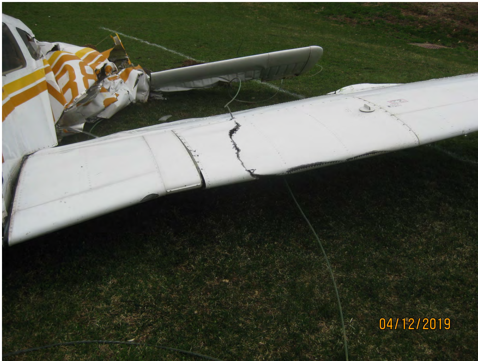
Photo 5 – Left wing damage (Photo courtesy of FAA)
