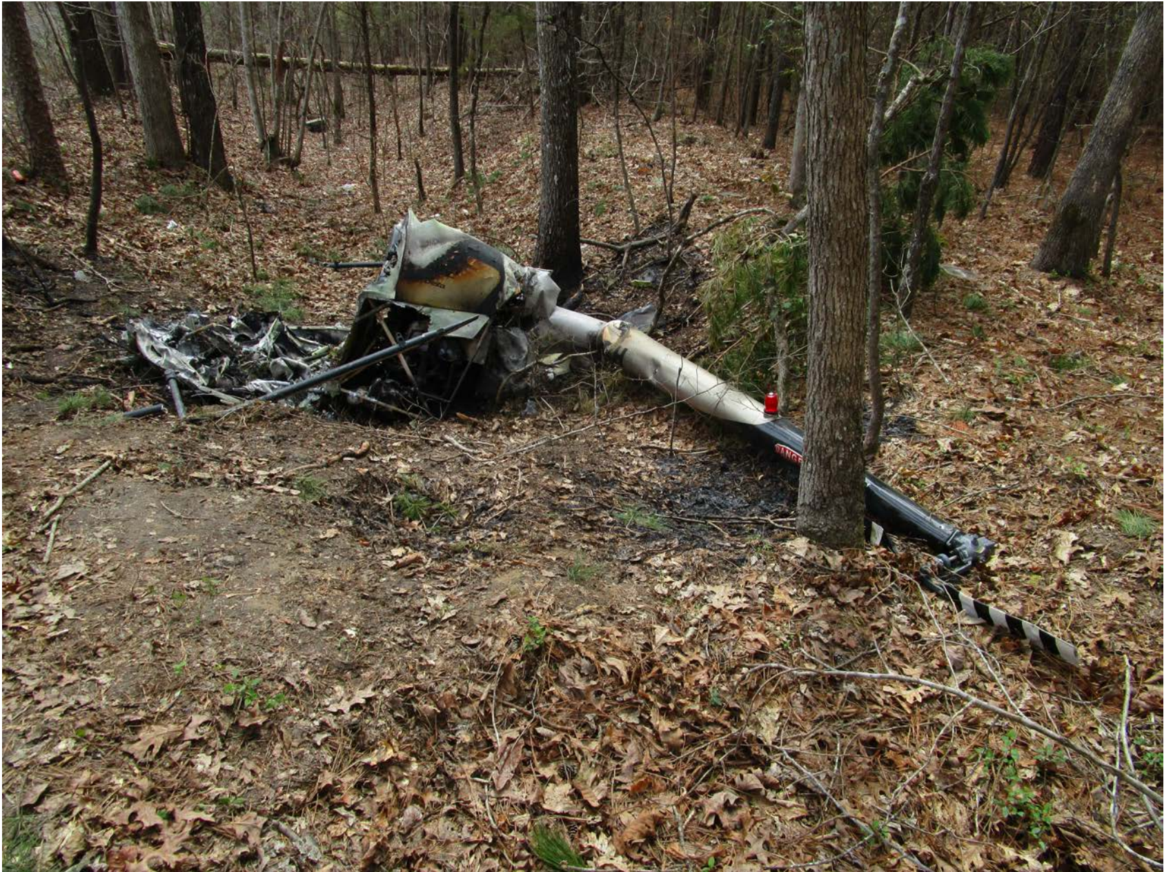
Photo 6 – View of tail boom and tail rotor showing buckling and post-crash fire damage
