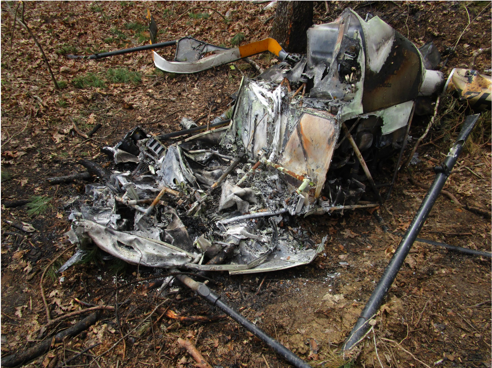
Photo 4 – Forward view of helicopter cabin section showing post-crash fire damage
