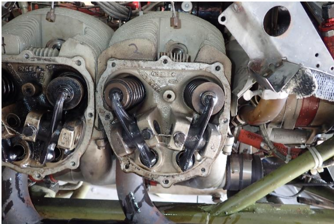
#2 Cylinder Overhead Components
