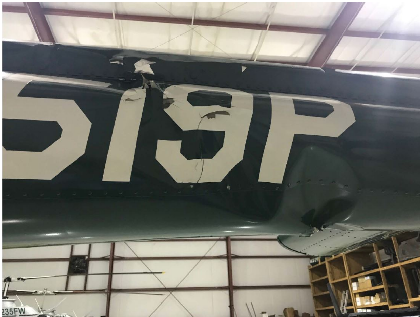
Tail boom Damage – View of Left Side (courtesy FAA)
