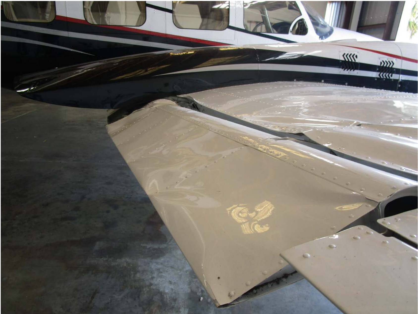
Photo 1 – View of top of inboard right wing showing buckling damage
