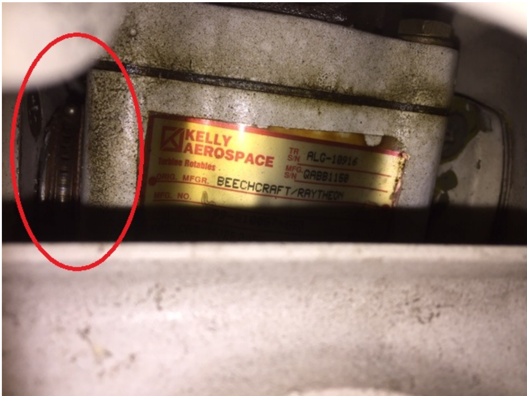
Photo 5 – Pinion Bearing separated from actuator (Mechanic)
