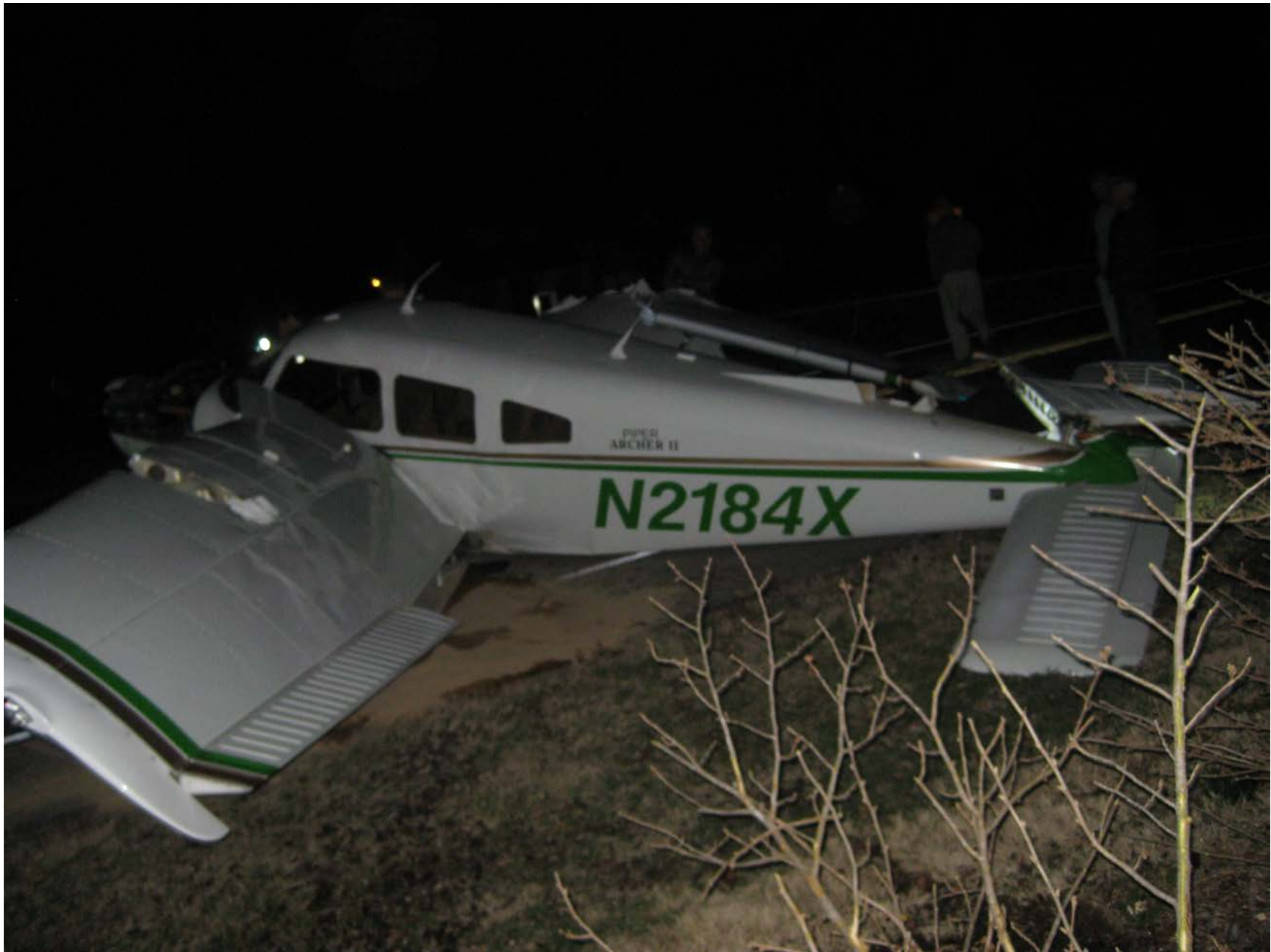
Photo 3 – View of left side of airplane showing vertical stabilizer damage
