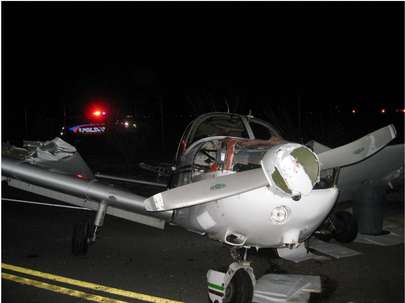
Photo 1 – View of front of airplane showing left wing damage
