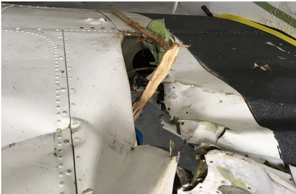
Figure 4: Right wing fracture close-up
