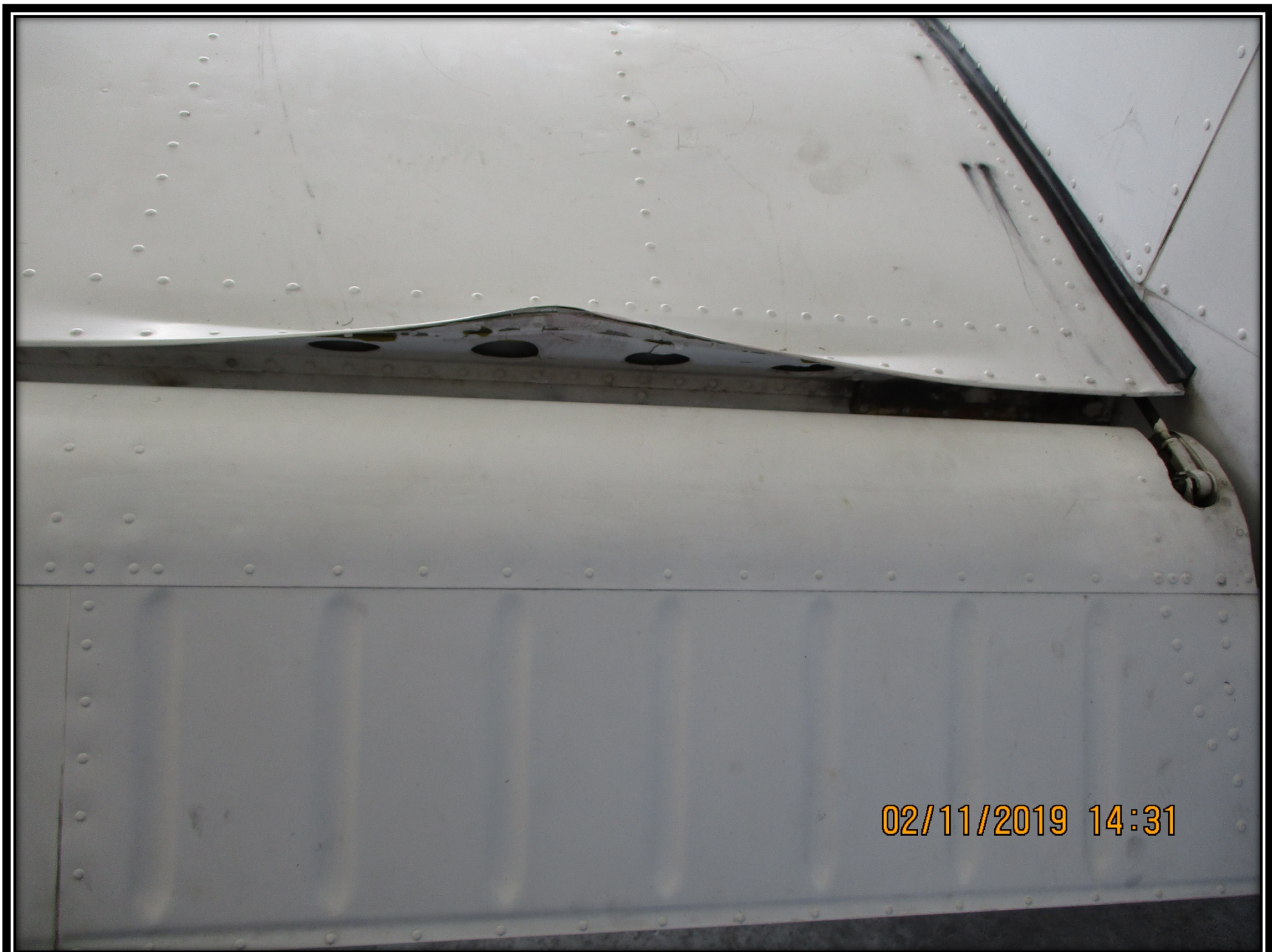
Photo 6 – Left Wing Trailing Edge (Photo Courtesy of FAA)
