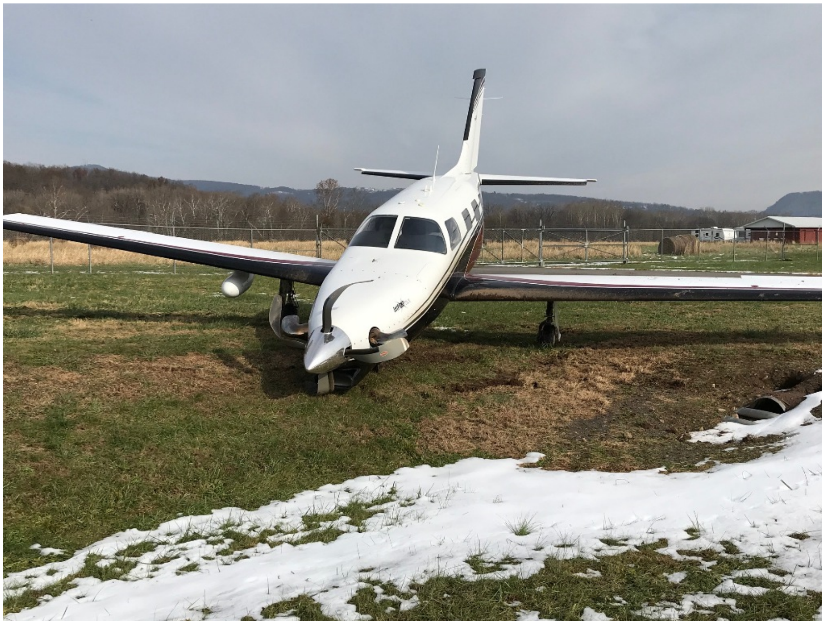
Photo 2 - FAA Digital Photograph. Frontal View of the Airplane Where it Came to Rest. Note the collapse Nose Landing Gear.
