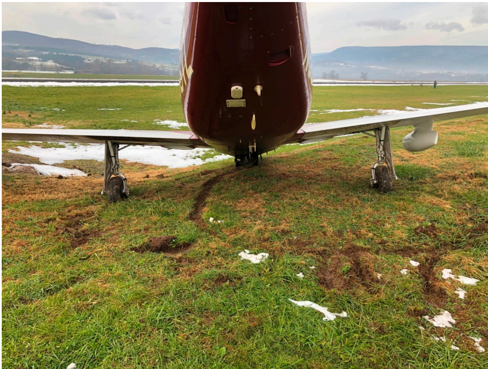
Photo 3 – Photograph From Pilot. View From Empennage Looking Forward. Note the Collapsed Nose Landing Gear.
