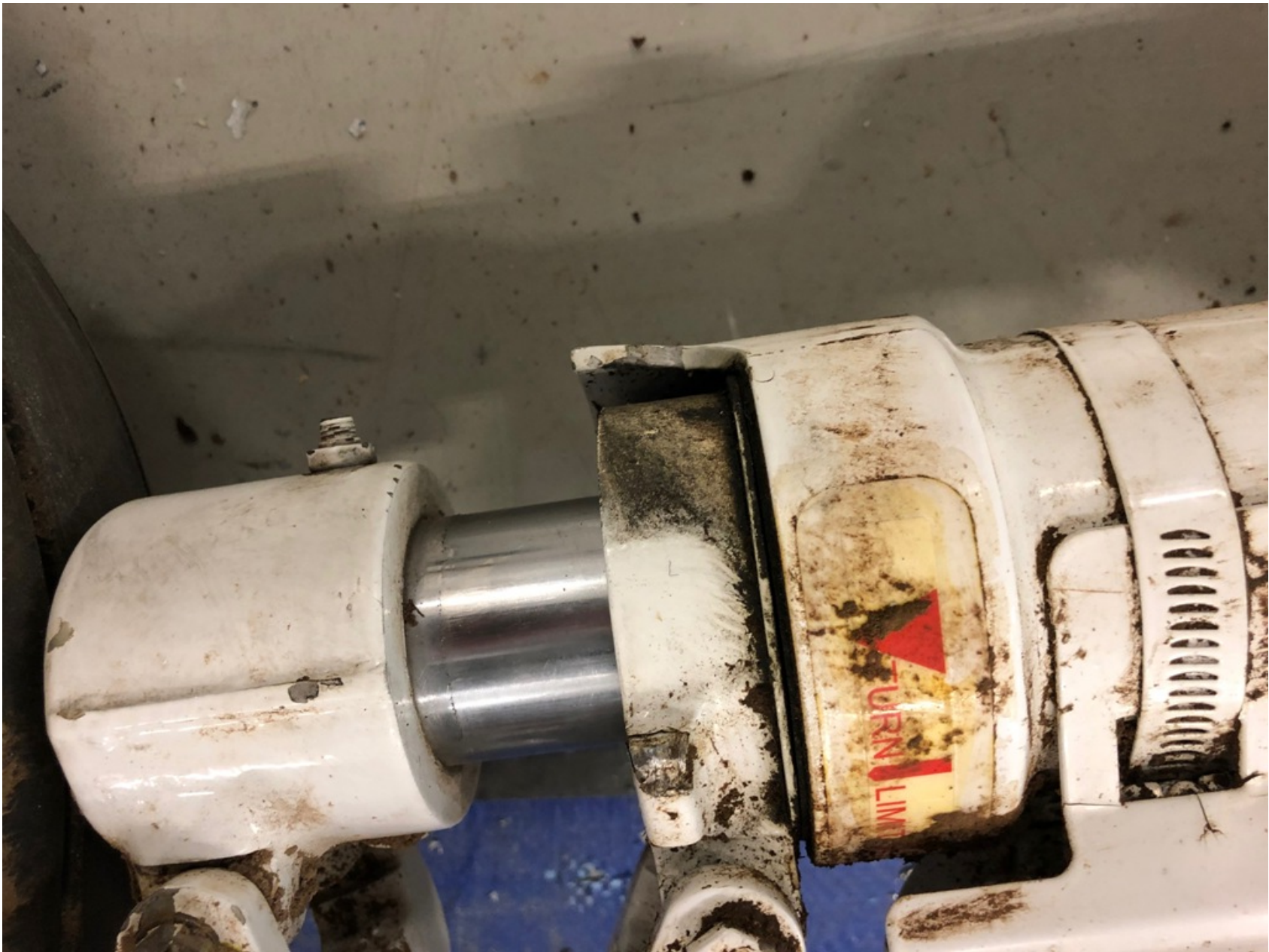
Photo 5 - Photograph From Pilot. View of the Damage to the Lower Portion of the Nose Landing Gear Trunnion Assembly.
