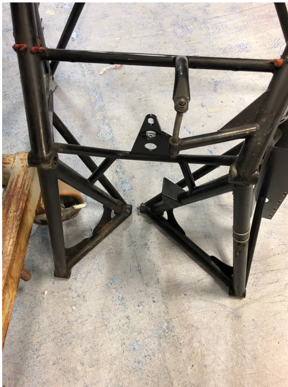
Photo 6 - Photograph From Pilot. View of the Engine Mount. Note the sheared bolt that Attached the Nose Landing Gear Actuator.
