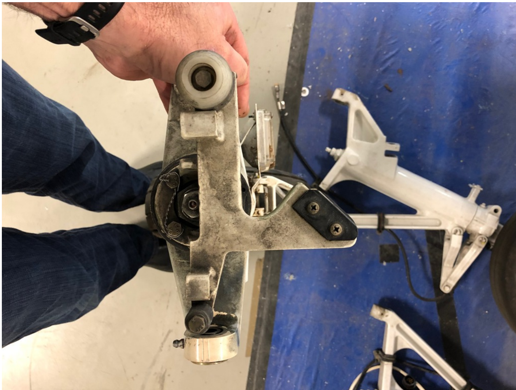
Photo 4 - Photograph From Pilot. View of the Upper Portion of the Nose Landing Gear Trunnion Assembly and Steering Horn.
