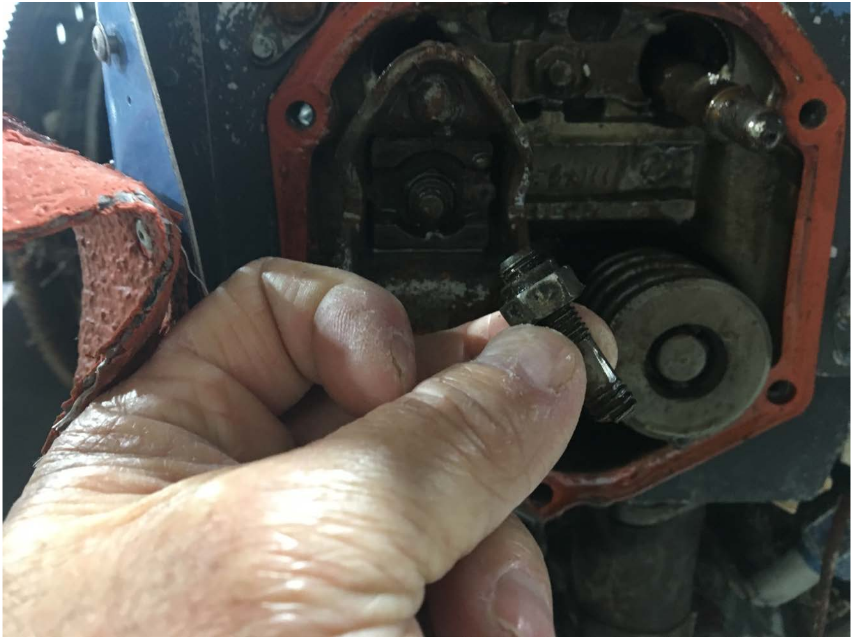
Photo 2 – Fractured Stud, exhaust rocker arm.
