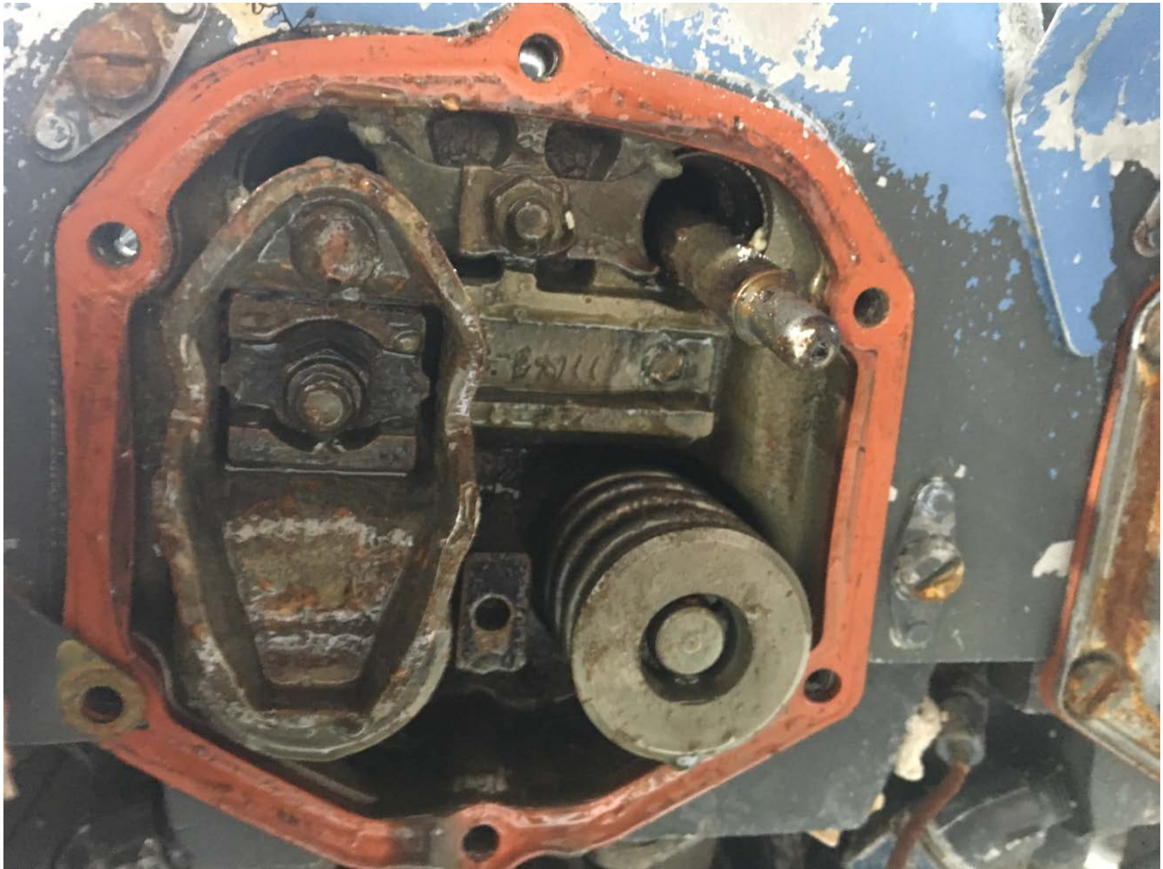
Photo 3 – No. 2 cylinder, fractured rocker arm stud.
