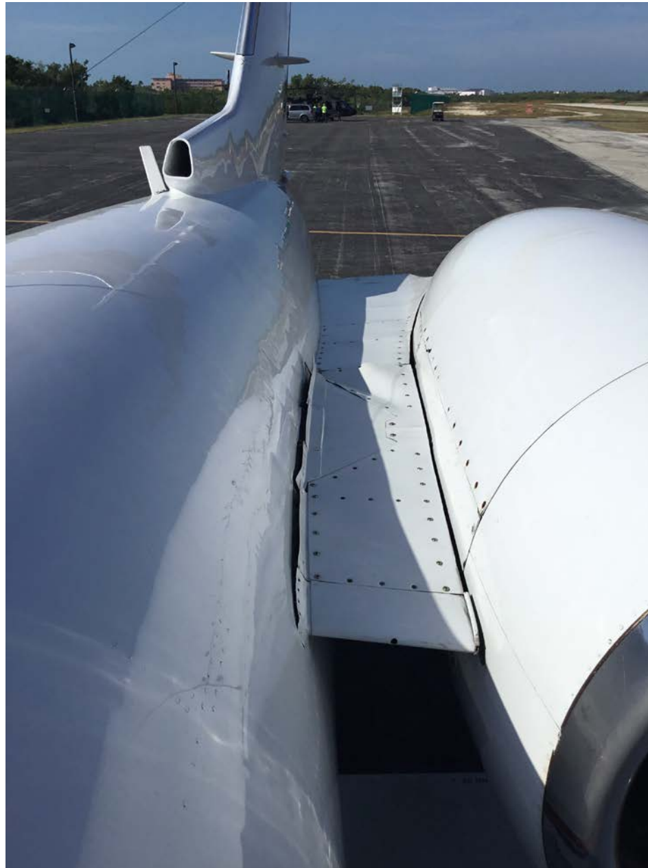
Photo 2 – View of damage to the left wing. (Photo courtesy of the FAA)
