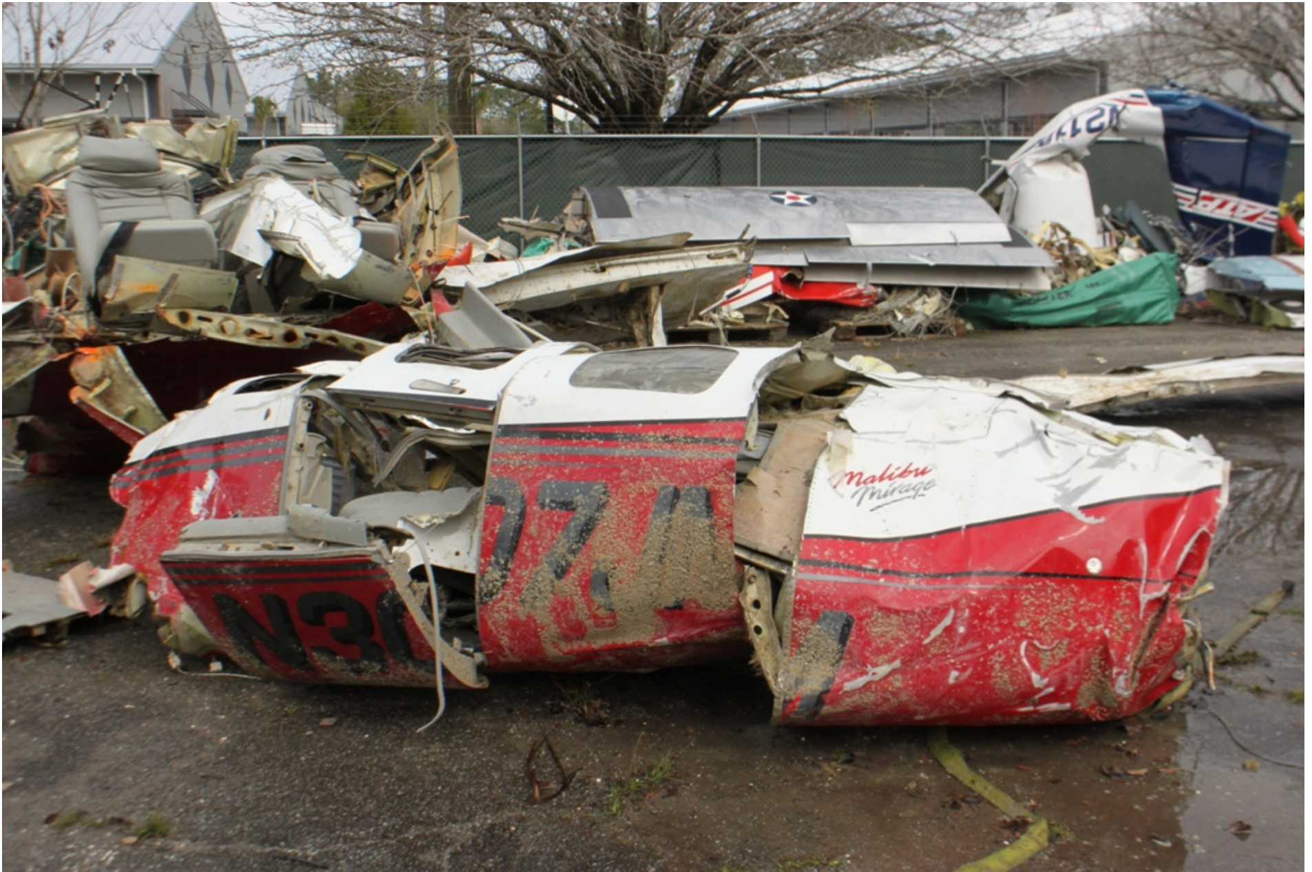
Photo 8 - NTSB Digital Photograph. View Depicting the Left Side of the Fuselage From the Aft Pressure Bulkhead Forward to Just Forward of the Cabin Entry Door.
