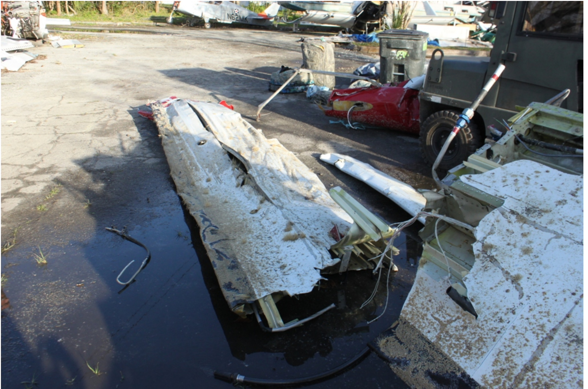
Photo 6 - NTSB Digital Photograph. View Depicting the Separated Outboard Section of the Right Wing.
