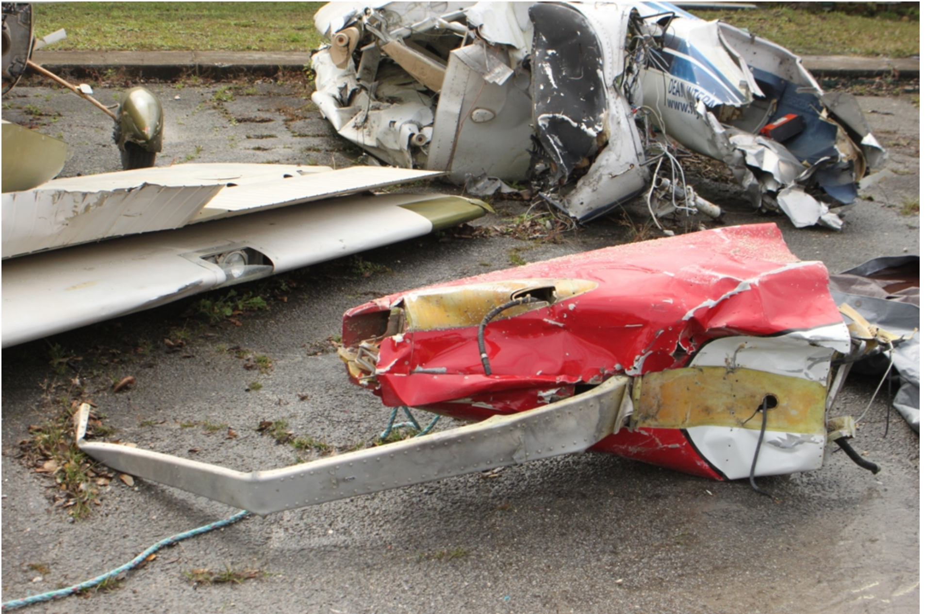
Photo 11 - NTSB Digital Photograph. View of the Aft Empennage Depicting the Vertical Stabilizer Aft Spar. Note the Separated Horizontal Stabilizer and Elevators, and Majority of the Vertical Stabilizer and Rudder.
