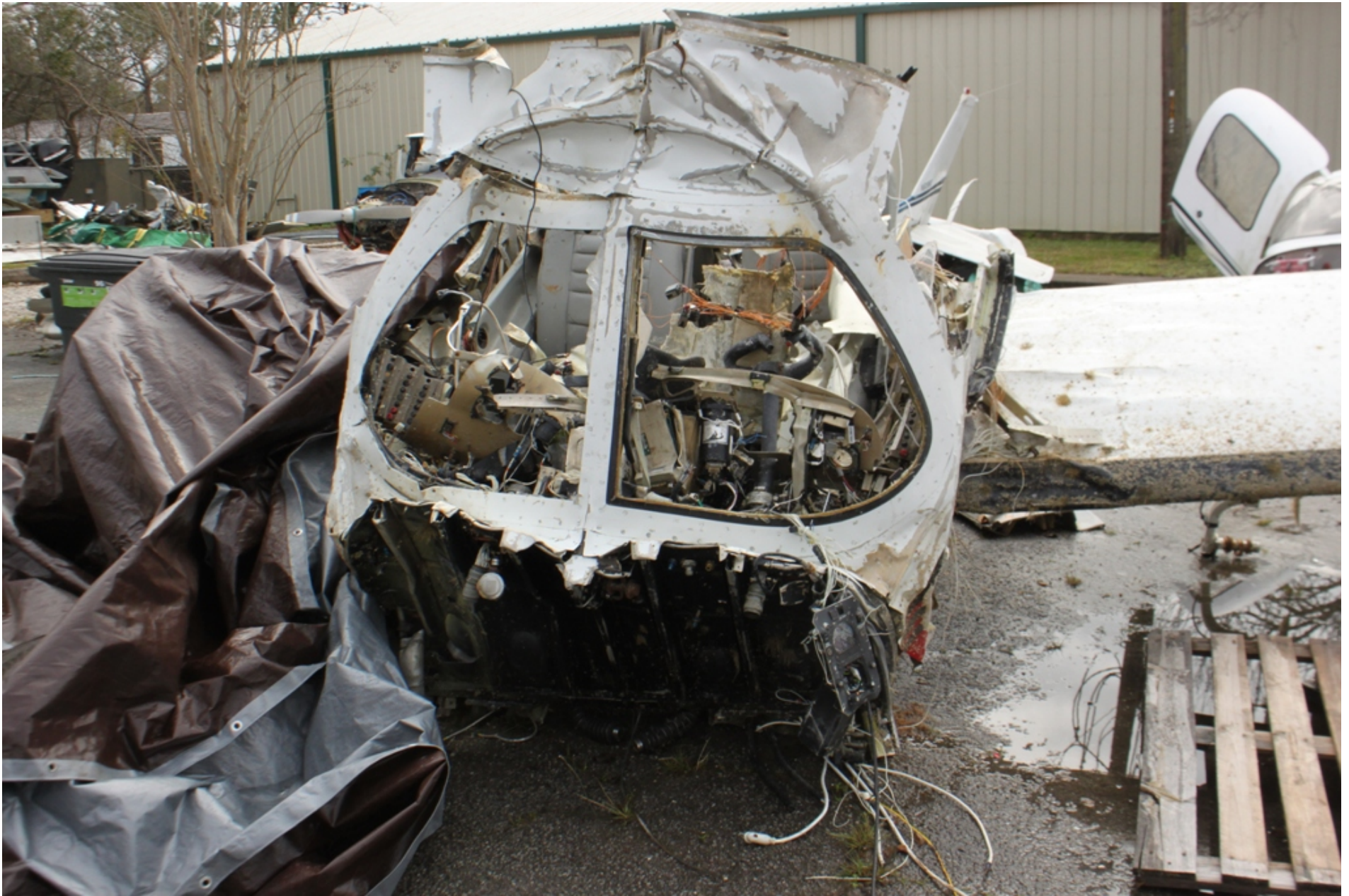
Photo 2 – NTSB Digital Photograph. Frontal View of the Fuselage and Inboard Section of the Left Wing Following Recovery. Note the Damaged/Missing Windscreens.
