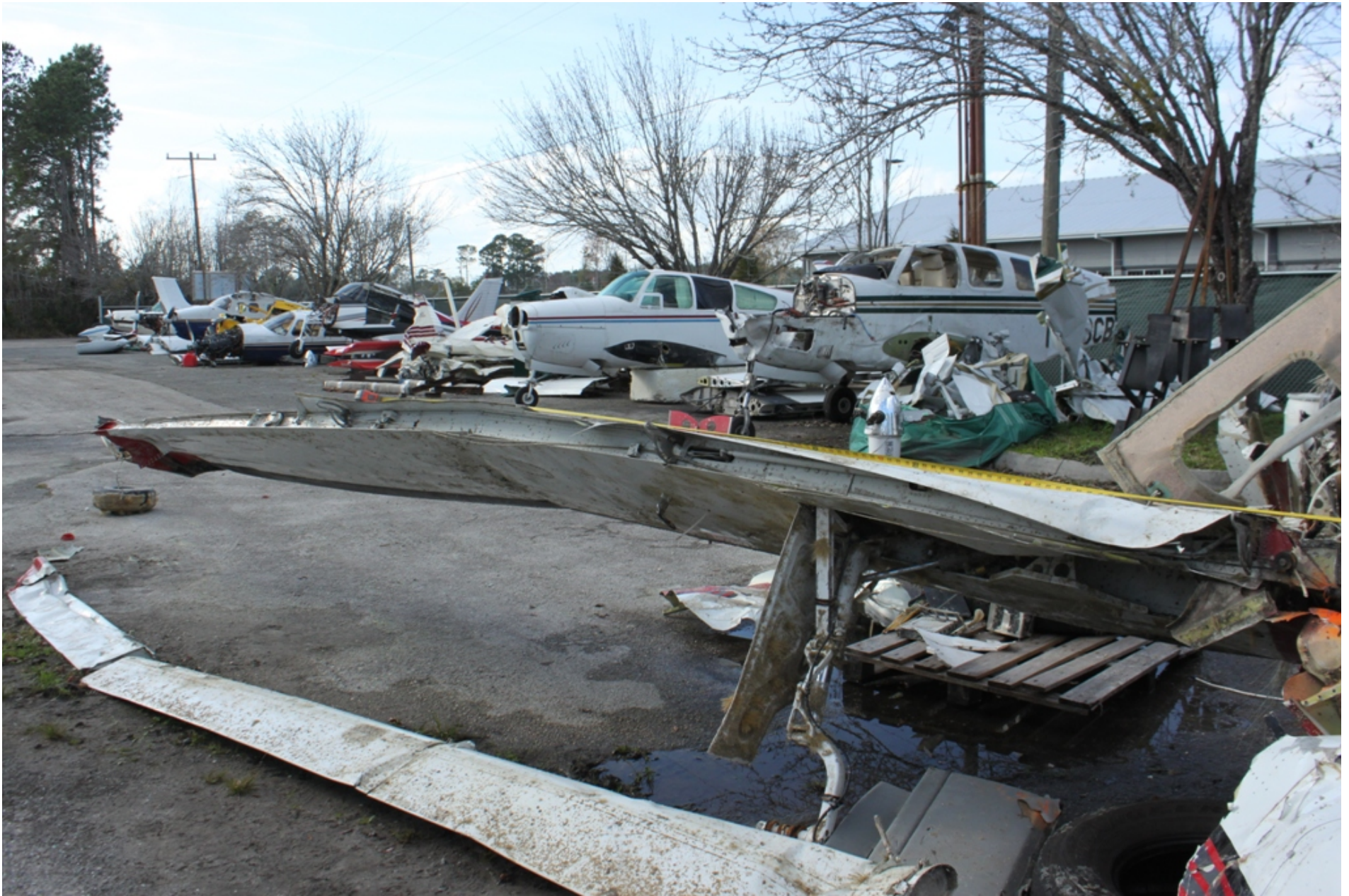
Photo 4 - NTSB Digital Photograph. View Taken Behind Left Wing Looking Forward. Note the Permanent Bow/Displacement of the Wing.
