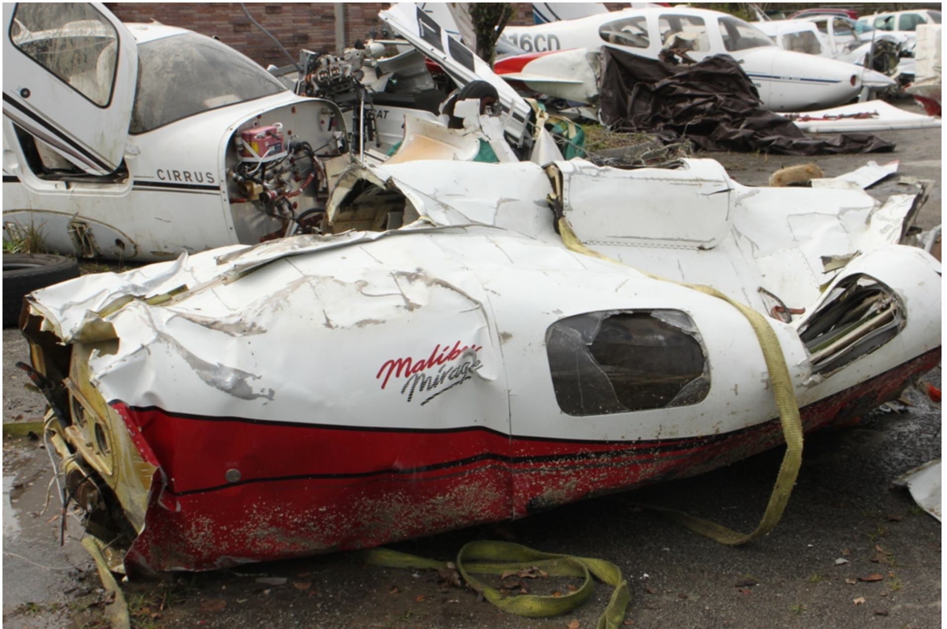
Photo 7 - NTSB Digital Photograph. View Depicting the Right Side of the Fuselage From the Aft Pressure Bulkhead Forward. Note the Down Crushing on the Fuselage Crown.
