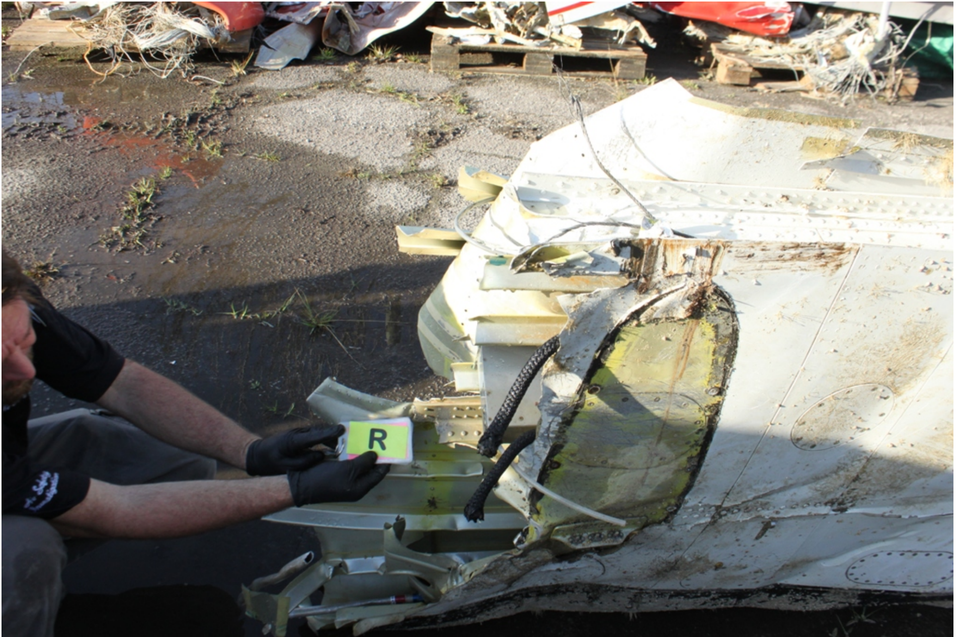
Photo 5 - NTSB Digital Photograph. View Depicting the Lower Portion of the Right Wing and the Wing Fracture. Note the Separated Radar Pod Location.
