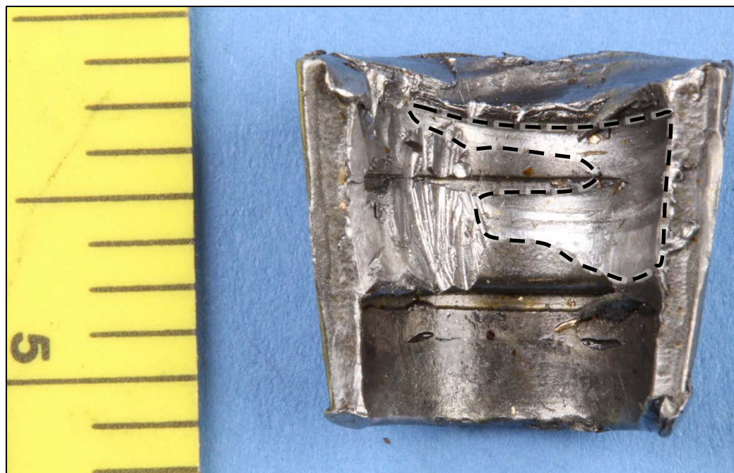
Figure 3. Interior face of one intake valve key. A dashed line indicates an area of smeared features with an off-axis cylindrical curvature matching the outer circumference of the intake valve tip.
