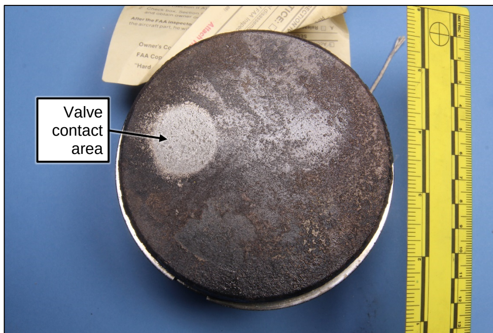
Figure 5. Piston crown showing a contact area that was generally free from combustion deposits.
