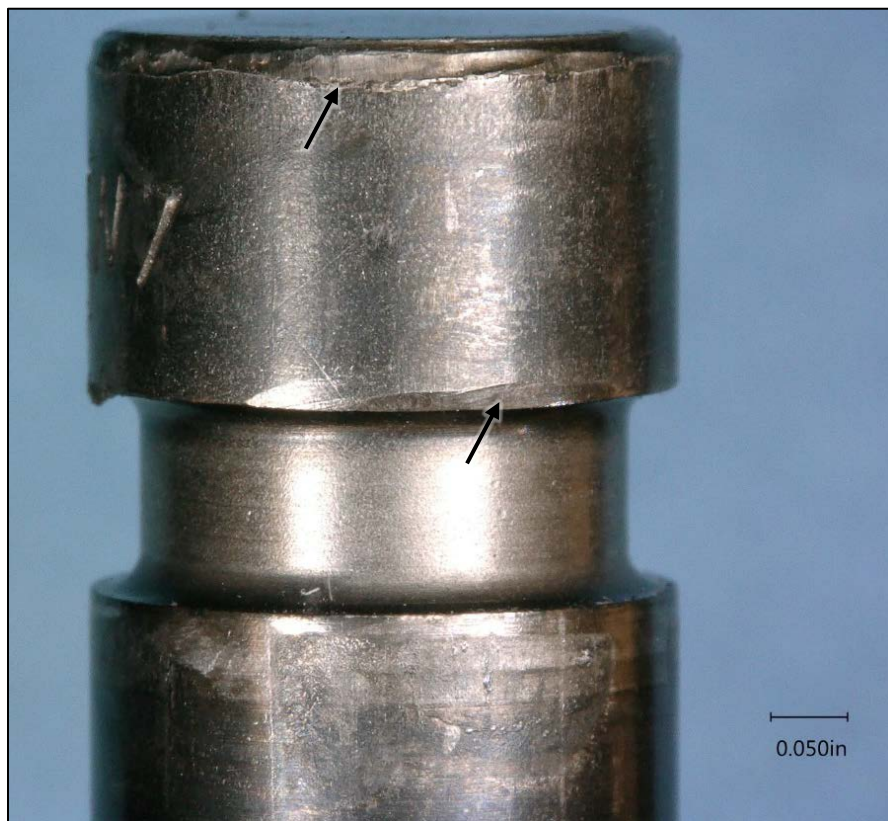
Figure 2. Intake valve tip. Unlabeled arrows indicate damage to the shoulder and the edge of the rocker contact face.
