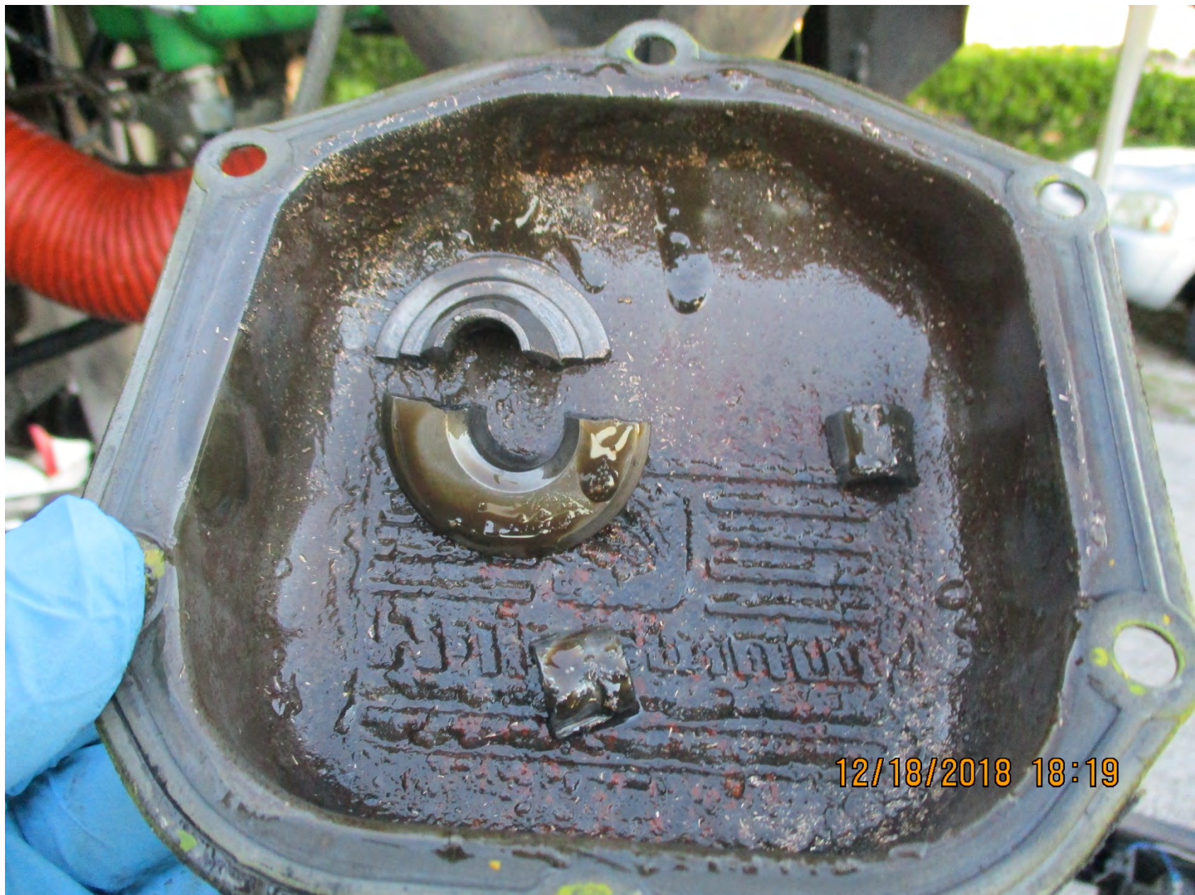
Photo 3 – No. 1 Rocker Cover, Broken Valve Spring Seat, Damaged Valve Key (Photo Courtesy of FAA)
