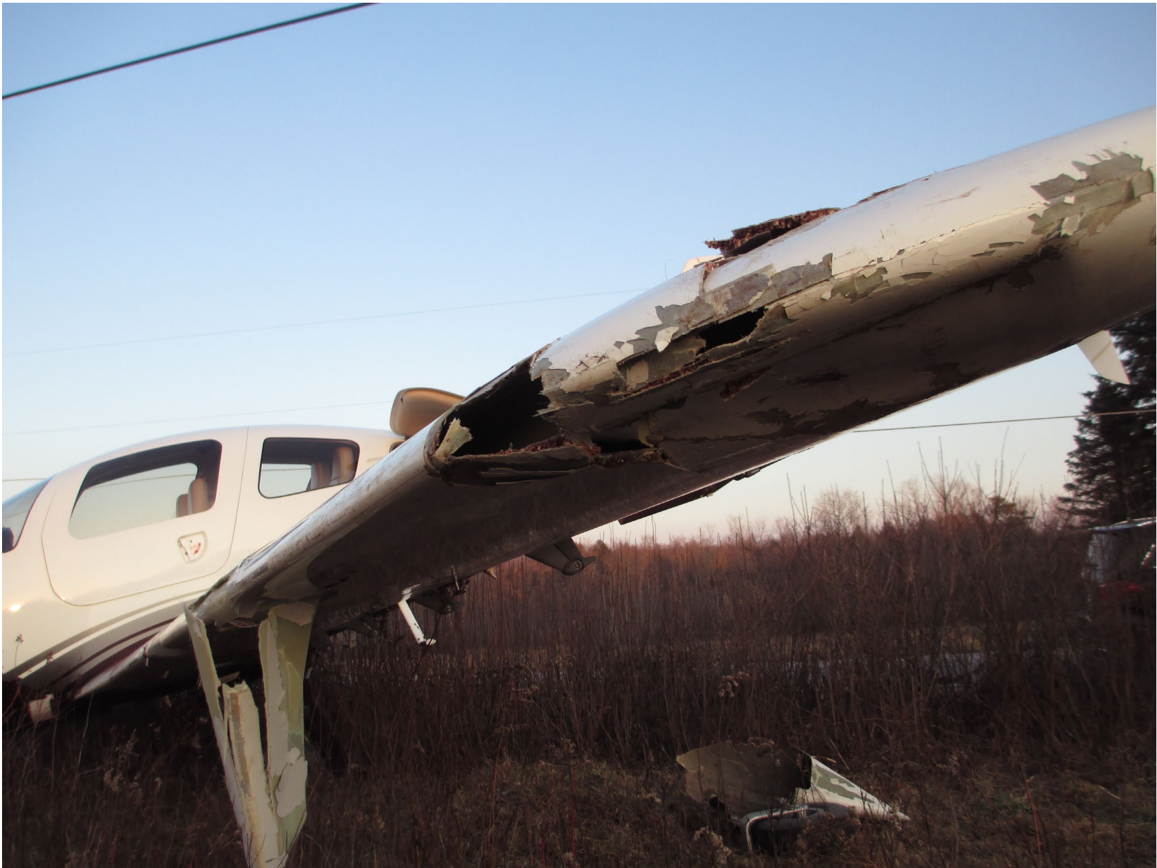
Photo 3 – View of the damage to the left wing. (Photo courtesy of the FAA)
