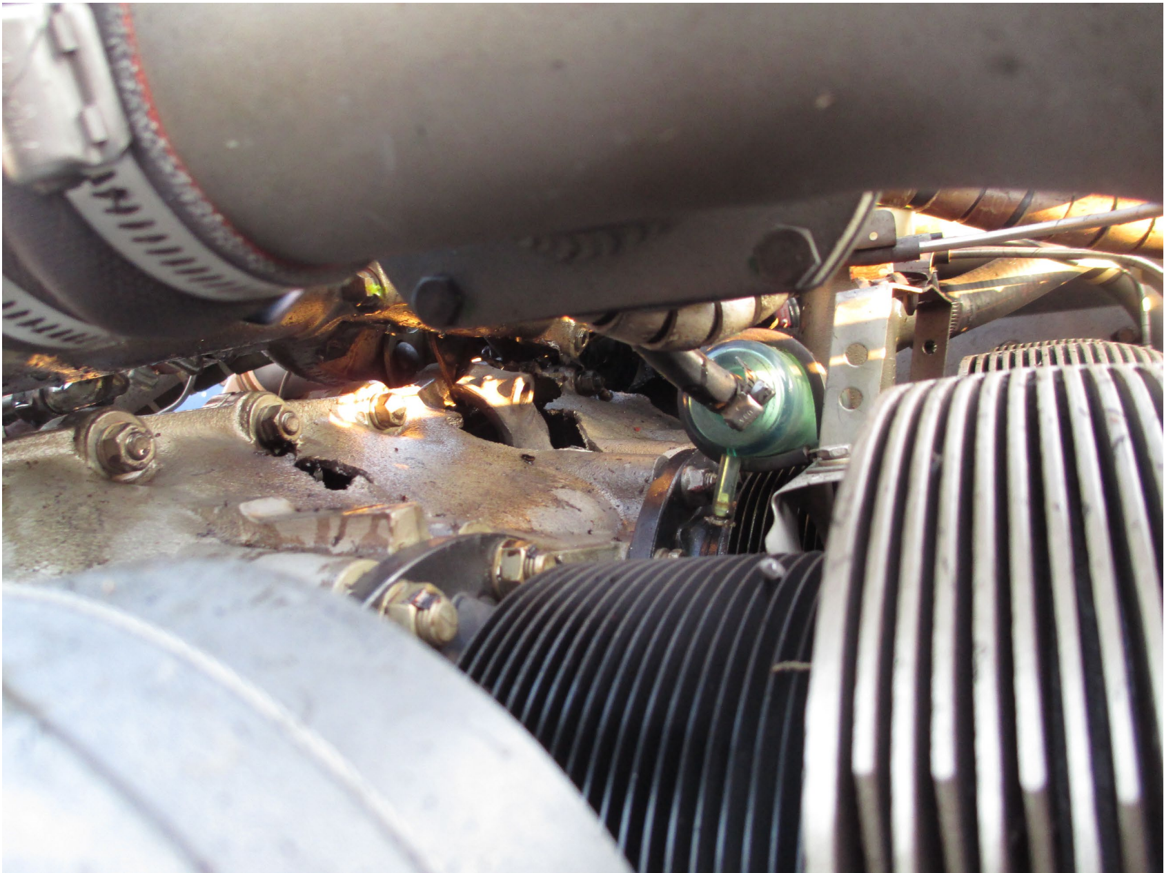
Photo 2 – View of the holes in the top of the crankcase. (Photo courtesy of the FAA)
