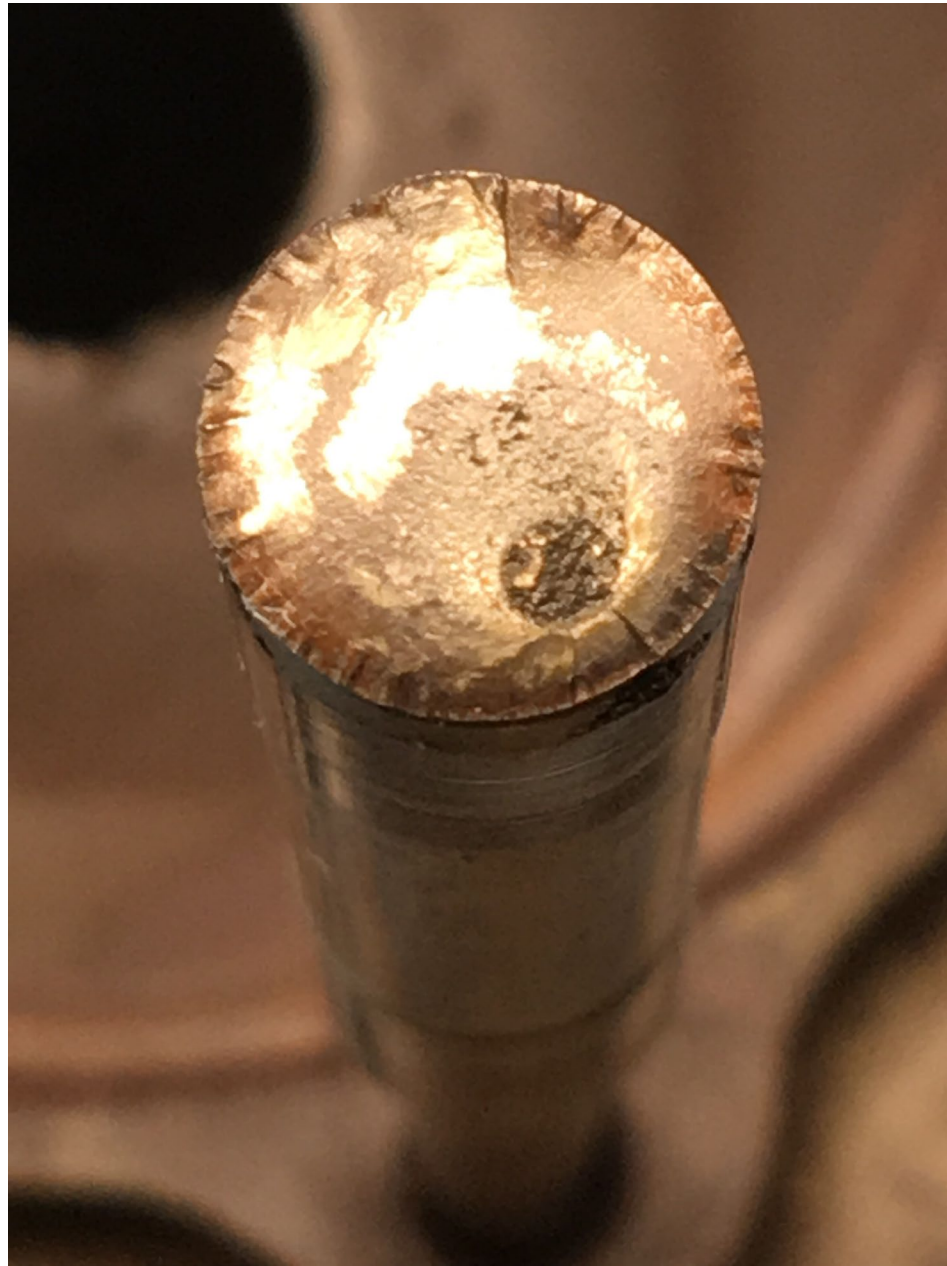
Photo 4 – View of the fracture surface of the turbo turbine wheel assembly shaft.
