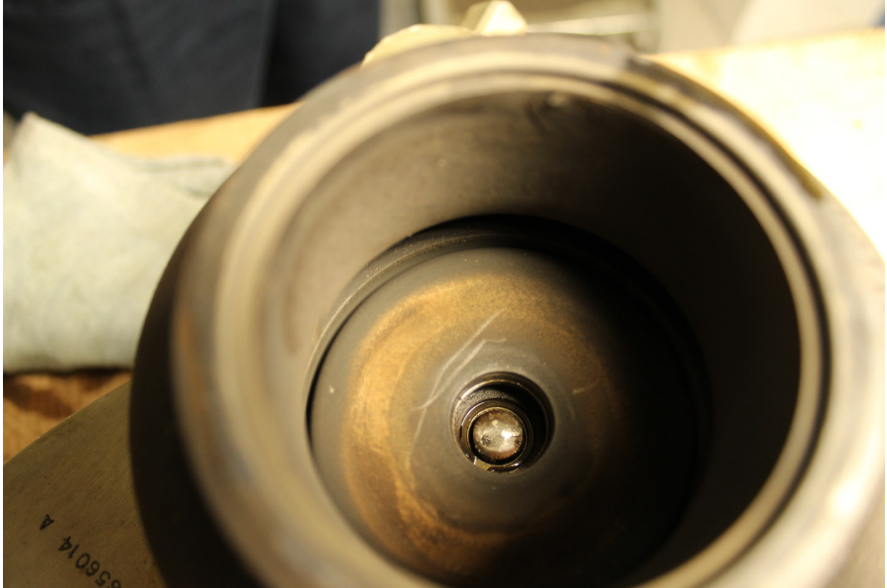
Figure 4: Missing turbine wheel from left turbo.
