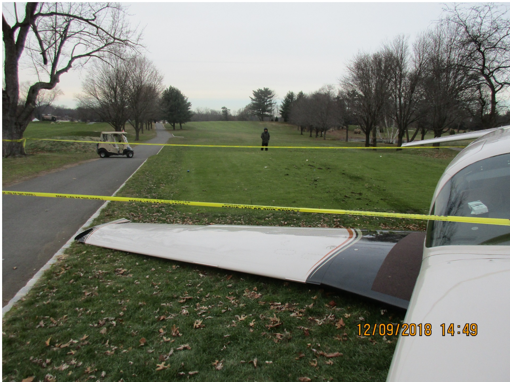
Photo 4 – View of wrinkled right wing (Courtesy of FAA)
