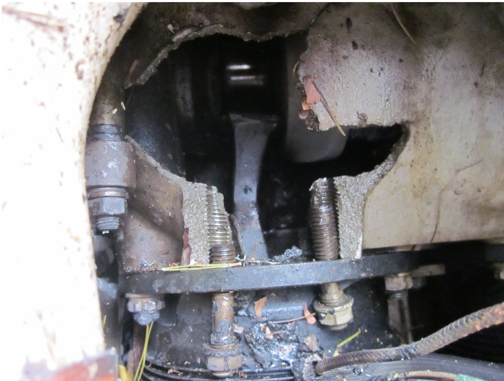
Photo 3 – Puncture of Engine Crankcase at the No. 6 Cylinder, as Viewed at the Accident Site (Photo Courtesy of FAA)
