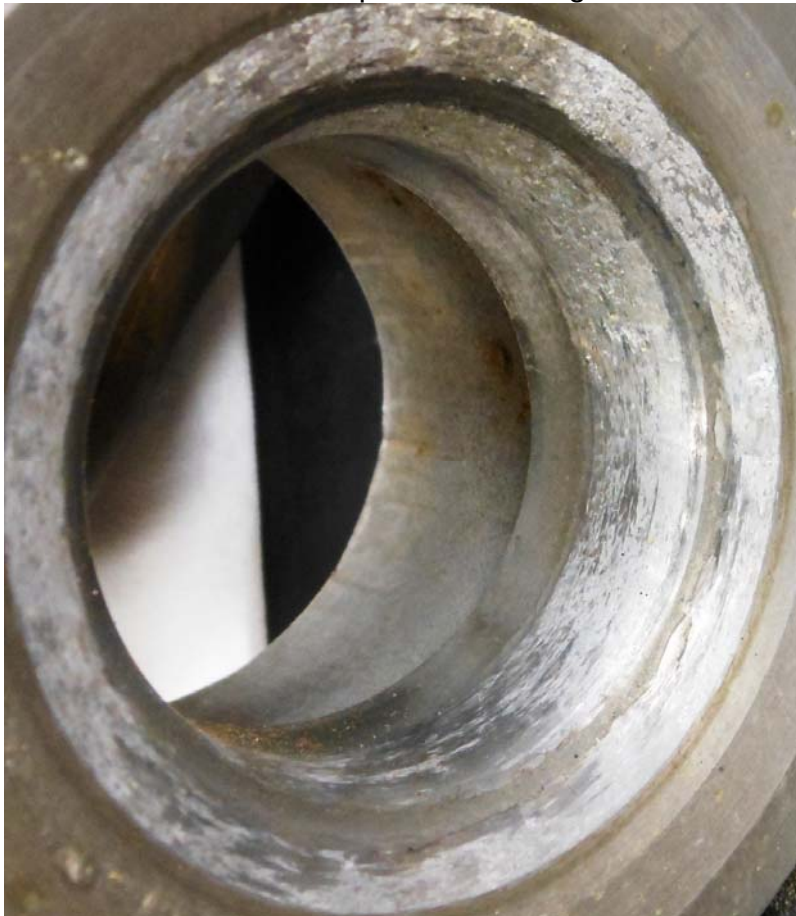
Photo #7 – Left compressor housing rub marks
