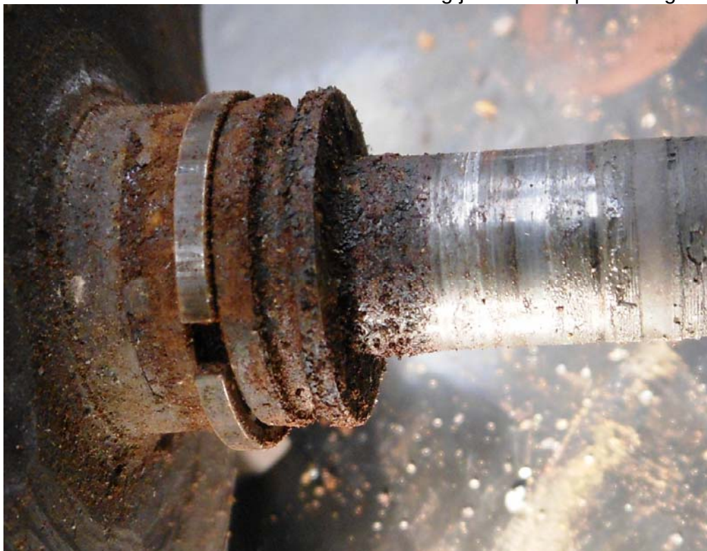
Photo #15 – Left shaft turbine-end bearing journal and piston ring
