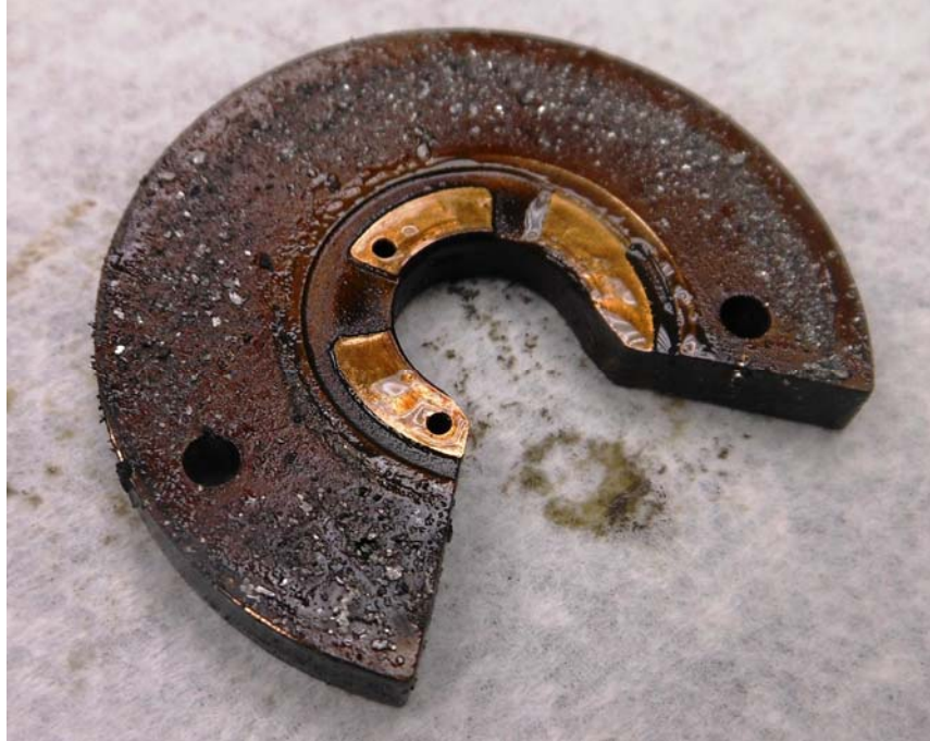
Photo #10 – Left thrust bearing with residual oil and aluminum particles
