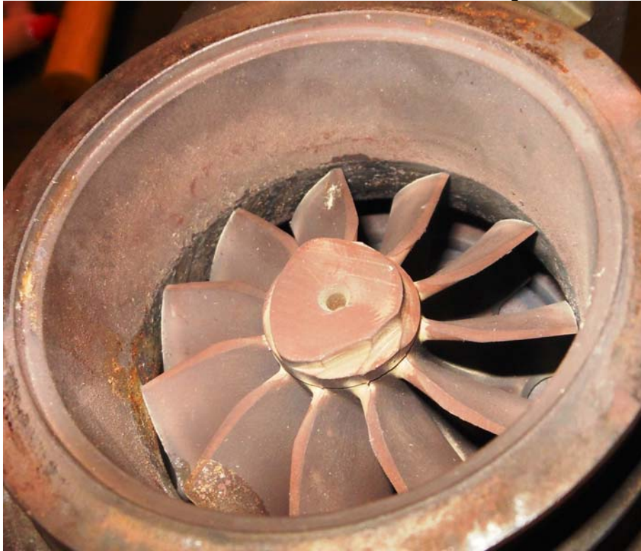
Photo #2 –Left turbine exit/wheel damage
