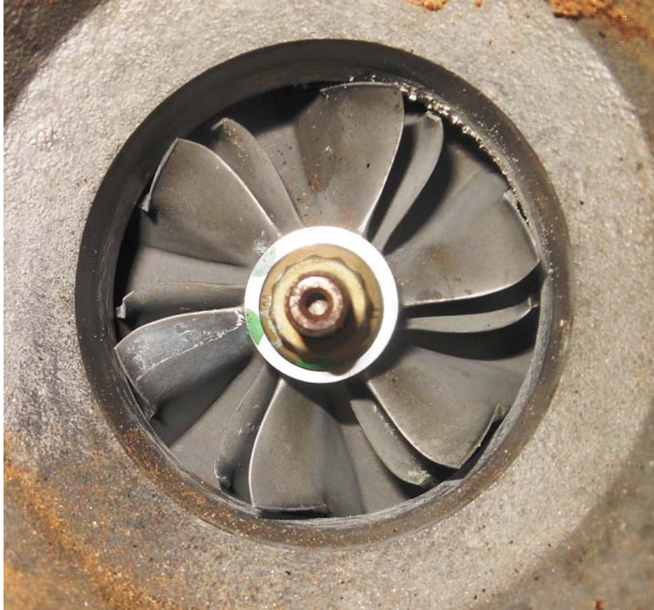
Photo #3 – Left compressor inlet/wheel damage
