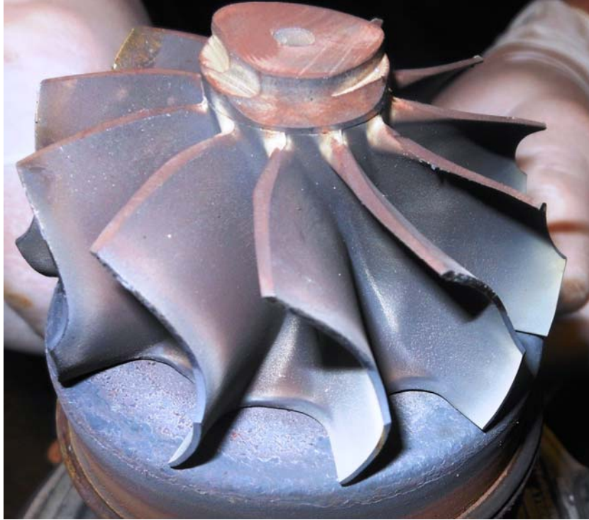
Photo #6 – Left turbine wheel and blade damage
