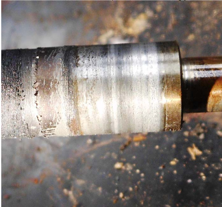
Photo #14 – Left shaft compressor-end bearing journal
