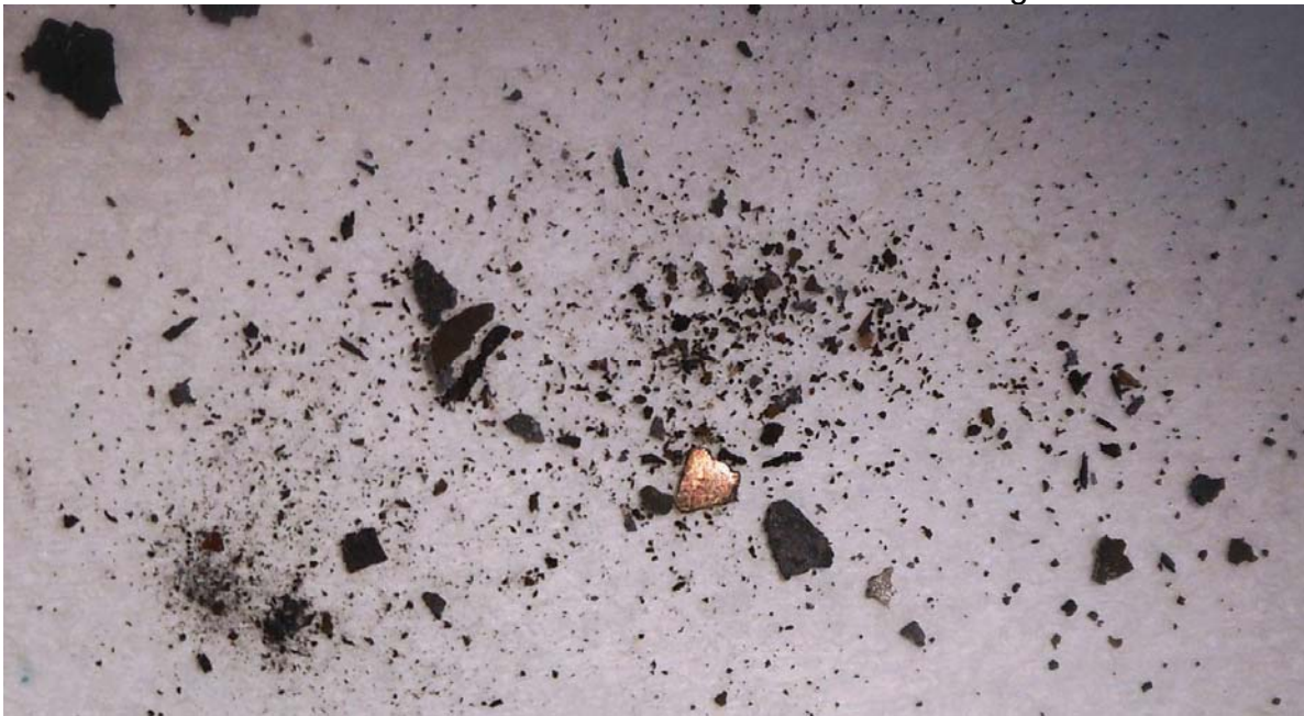
Photo #4 – FOD/debris from left turbine housing
