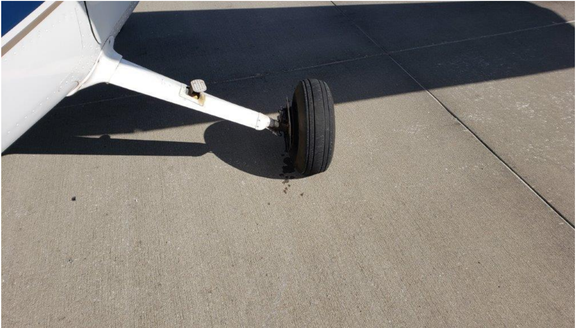
Photo 5 - FAA Digital Photograph. View Depicting The Right Wheel Assembly and Leaking Fluid Beneath the Right Brake.
