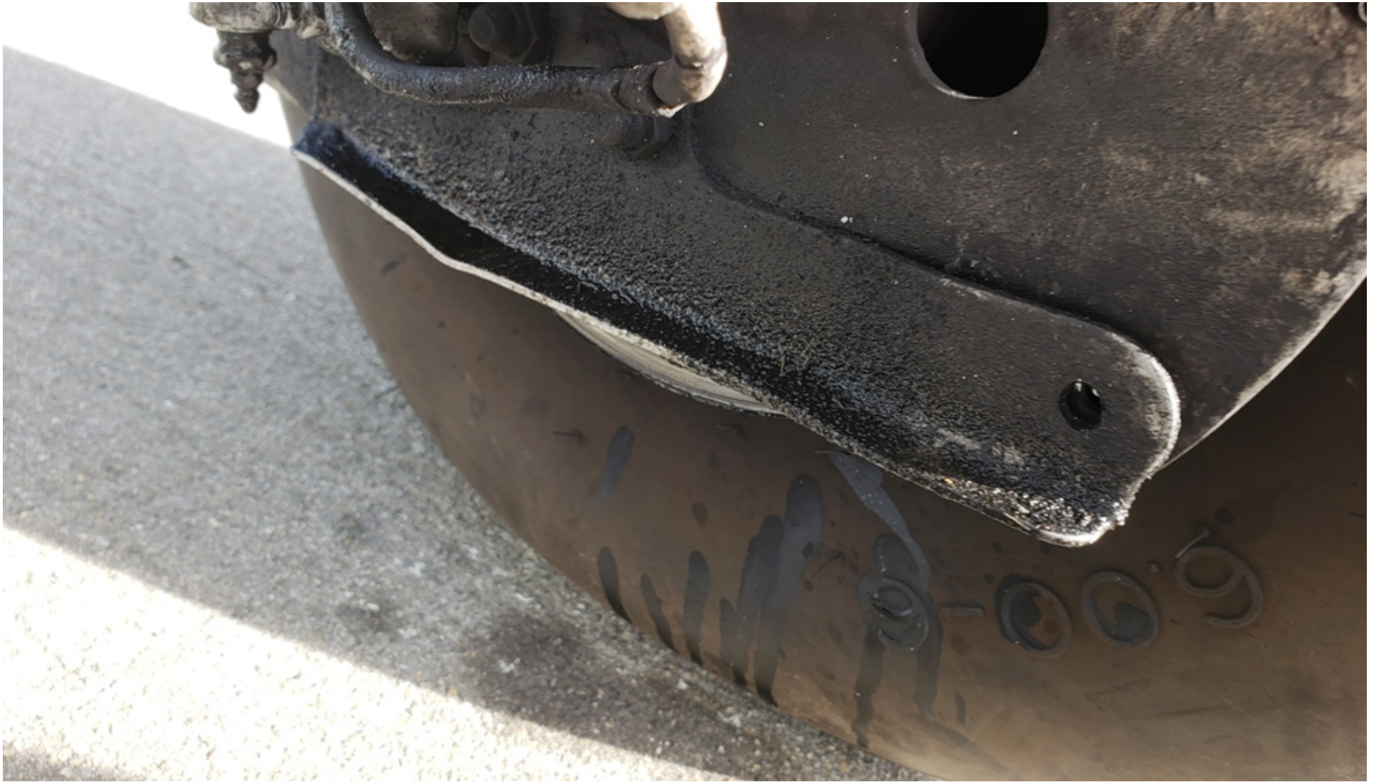
Photo 6 - FAA Digital Photograph. Close-Up View of the Lower Portion of the Right Main Landing Gear Tire Depicting Leaking Fluid from the Right Brake.
