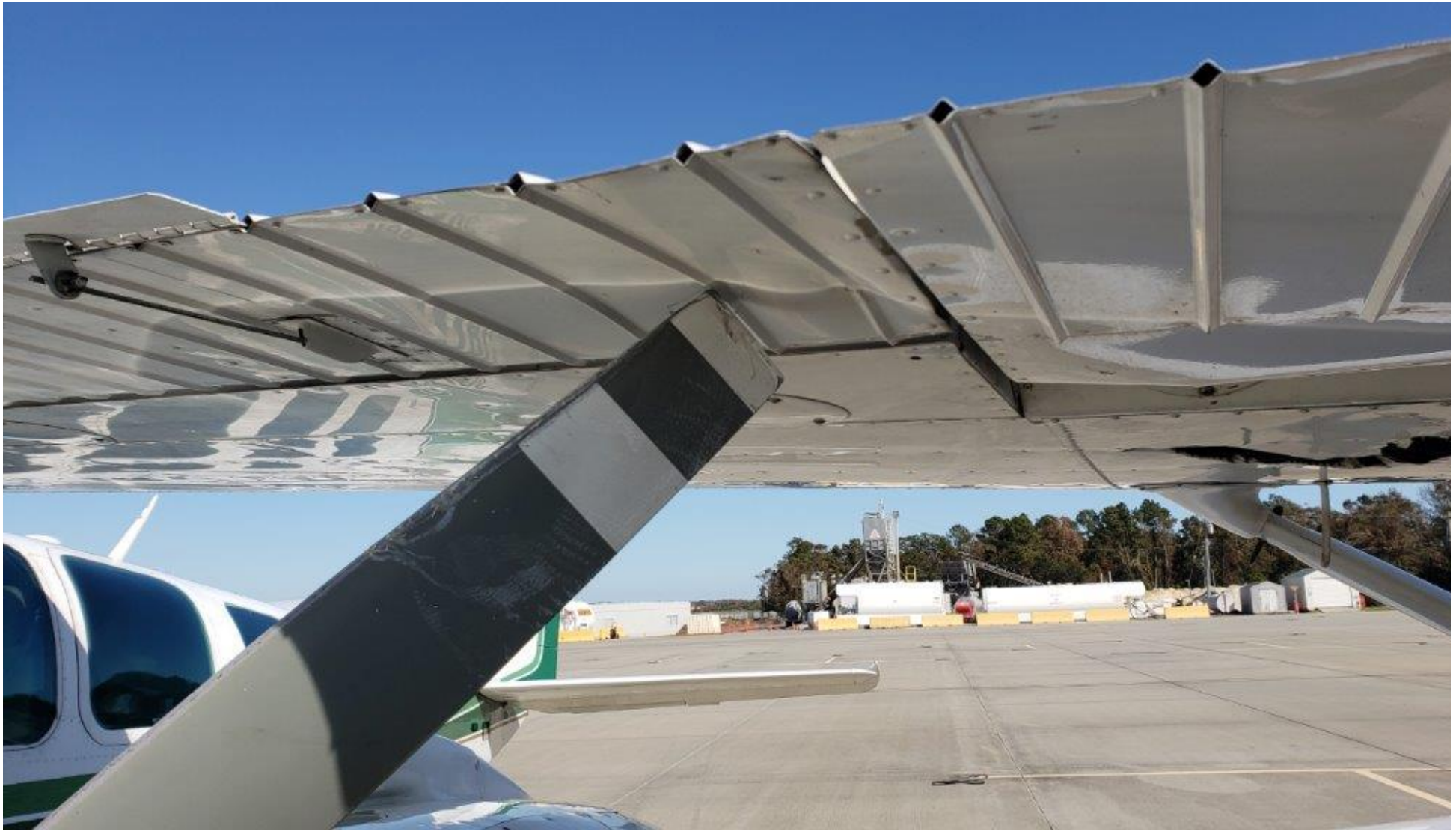
Photo 3 - FAA Digital Photograph. View Depicting The Damage to the Left Lower Wing Skin and Aileron of Accident Airplane.
