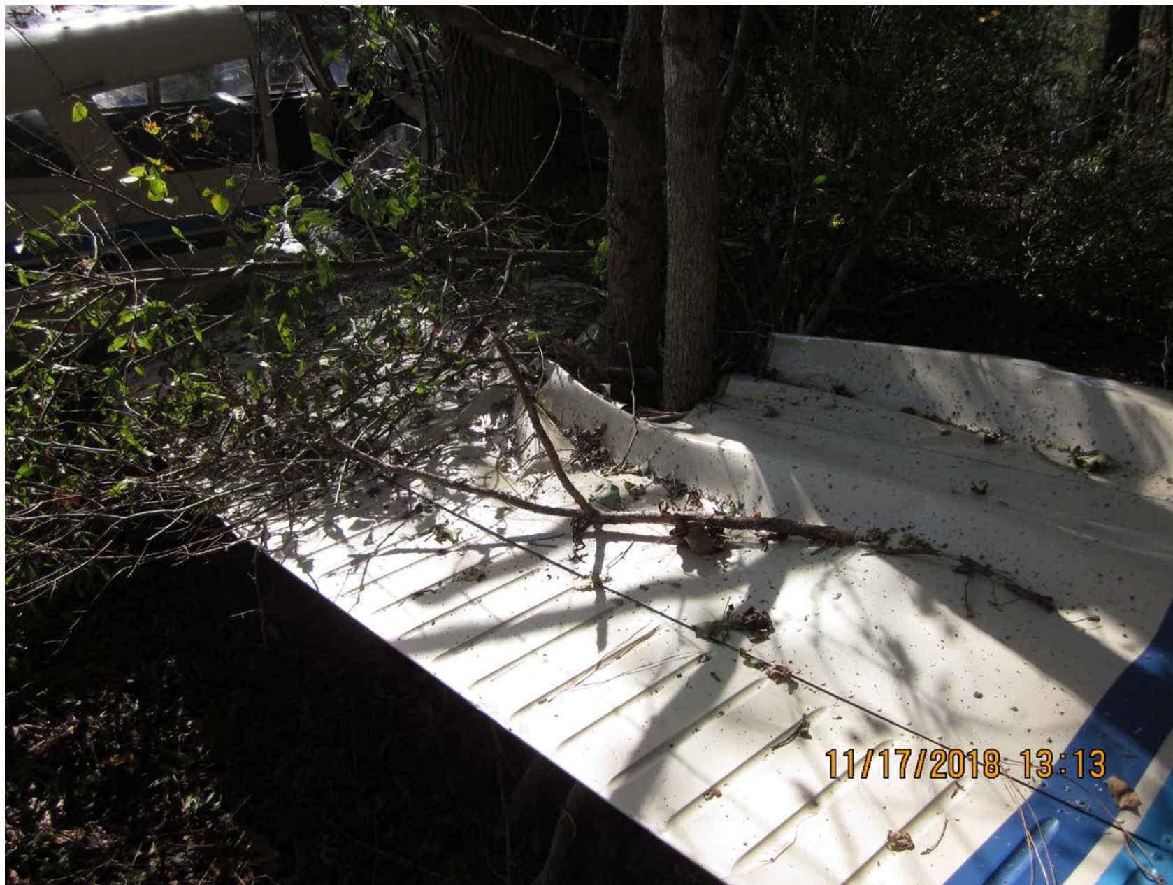
Photo 2 – Right Wing Damage (FAA Photo)
