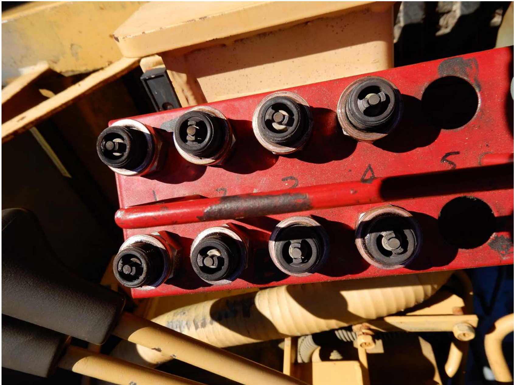
Photo 5 – Spark Plugs (NTSB Photo)
