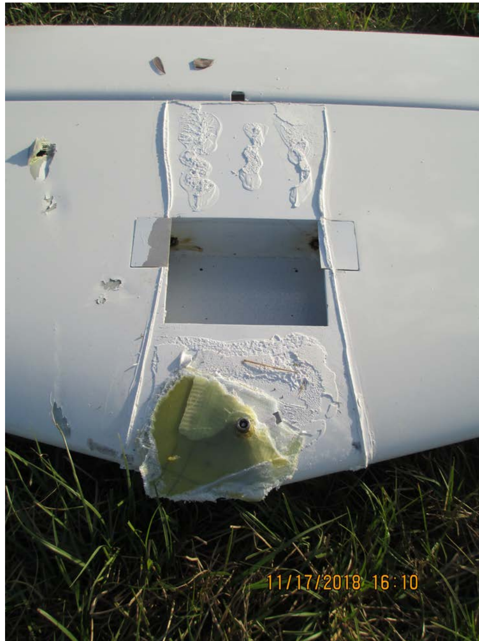
Photo 4 – View of Separated Horizontal Stabilizer with Fractured Tailcone Structure Attached (FAA)
