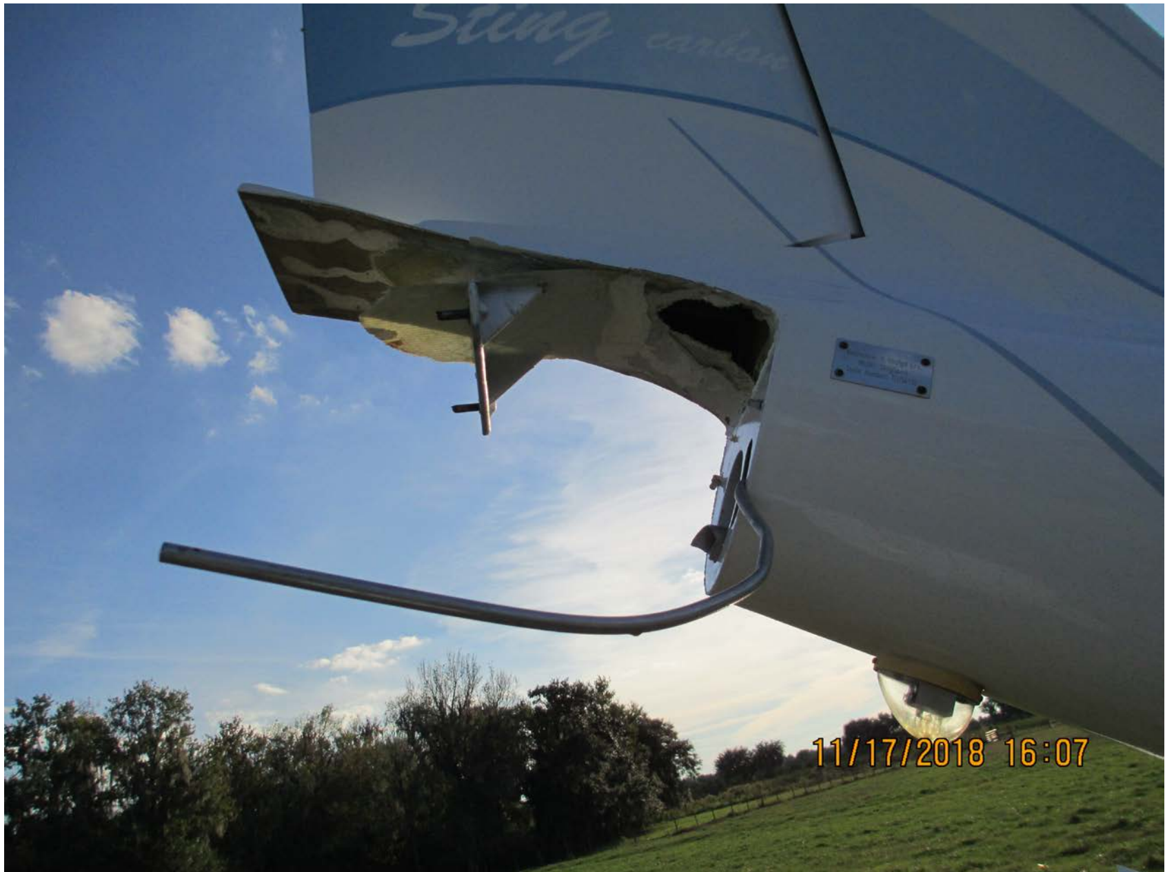
Photo 3 View of Fiberglass Delamination and Hole in Empennage Tailcone (FAA)-
