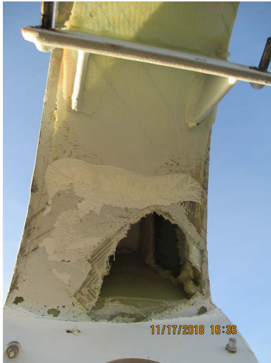
Photo 5 – View of Fractured/Separated Tailcone Structure (FAA)
