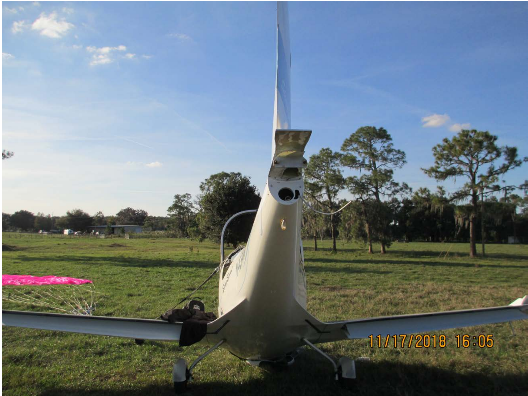
Photo 2 – View of Fractured Horizontal Stabilizer Mount (FAA)
