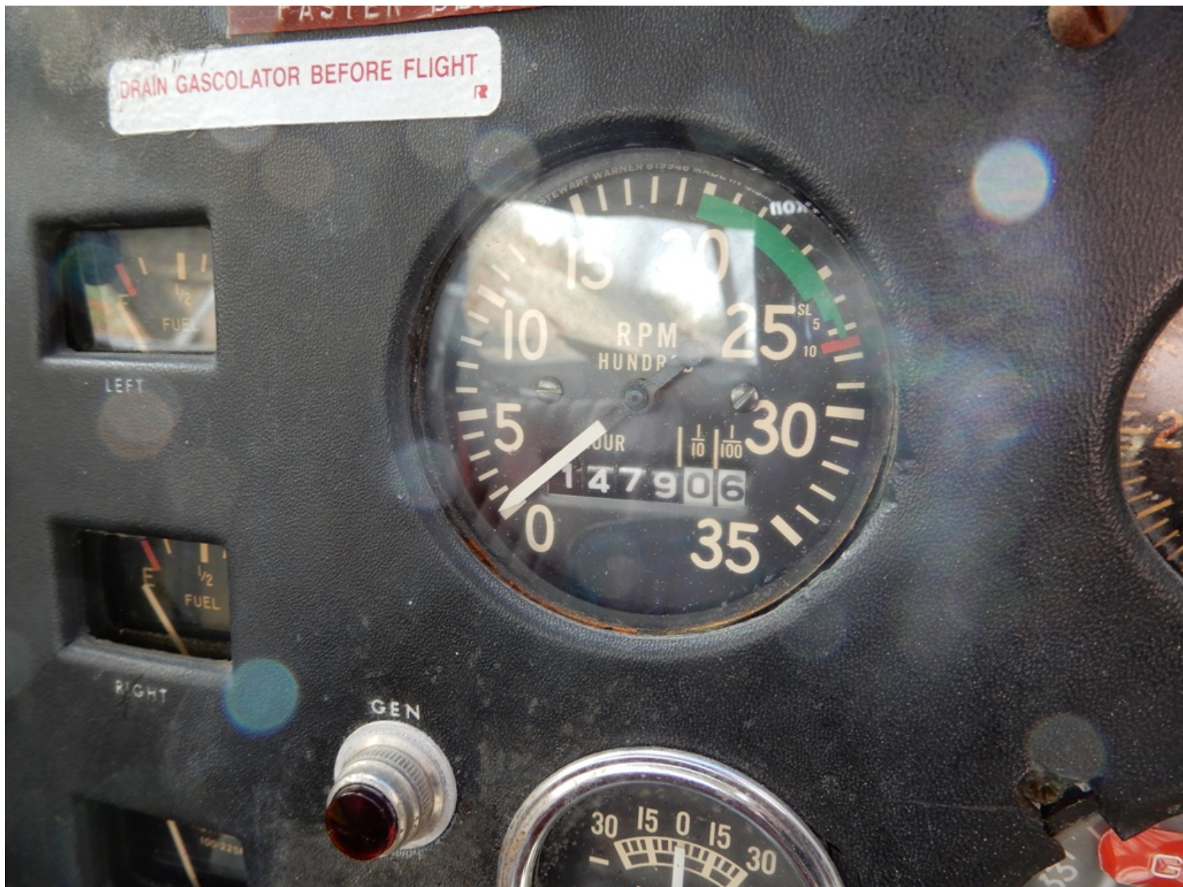
Photo 5 – Hour Meter (NTSB Photo)
