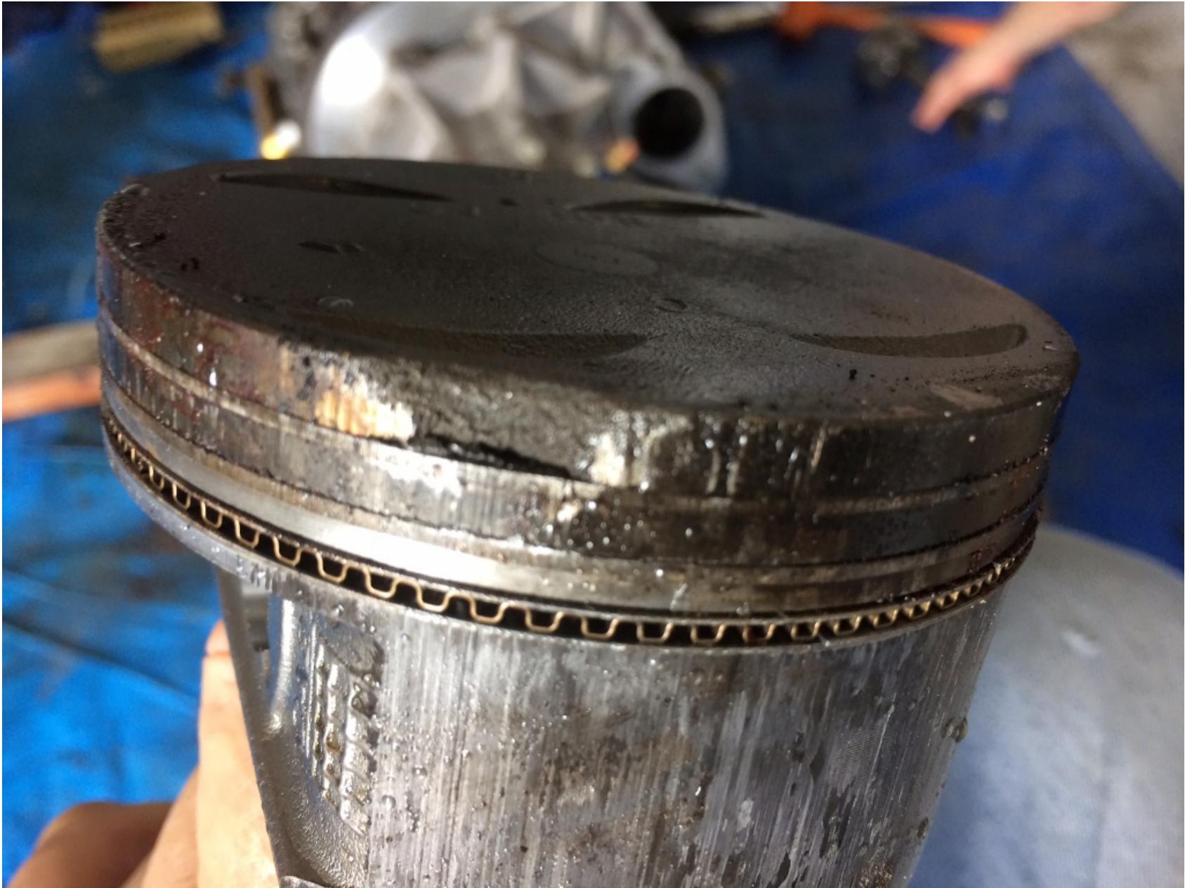
Photo 3 - Photograph From Owner/Builder. View of the Damaged No. 2 Piston. Note the course Scoring on the Side of the Piston and the Missing Section of Piston Crown.
