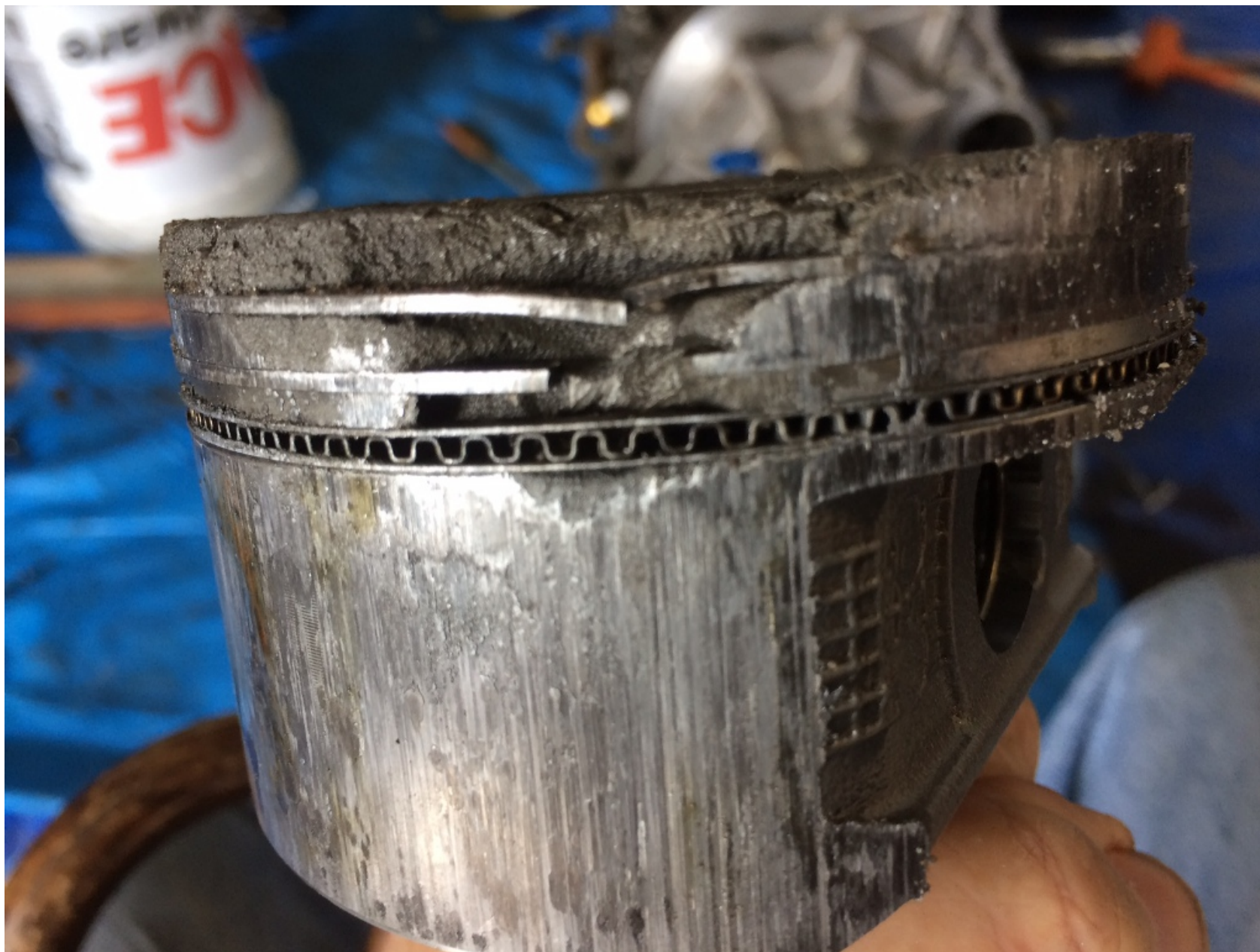
Photo 4 - Photograph From Owner/Builder. View of the Damaged No. 5 Piston. Note the course Scoring on the Side of the Piston, Missing Section of Piston Crown, and Damaged Piston Ring Lands.
