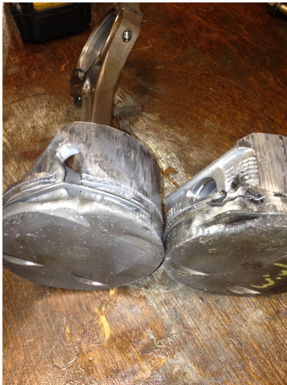
Photo 5 – Photograph From Owner of Similar Airplane With Same Engine. View Depicting Damage to Pistons. Note Damage to the Ring Lands and also Course Scoring on the Sides of the Pistons.
